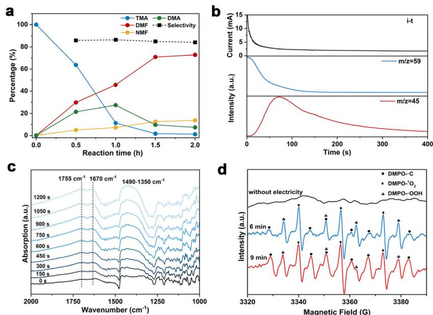
**Fig. 2** (a) Time-dependent conversions of TMA in 0.7 M  $K_2CO_3$ . (b) DEMS results at 1.1 V vs. Hg/HgO in 0.7 M  $K_2CO_3$  with 20 mM TMA. (c) *In situ* IRRAS of the reaction in 0.7 M  $K_2CO_3$  with 20 mM TMA at 1.1 V vs. Hg/HgO. (d) EPR spectra of the reaction in 0.7 M  $K_2CO_3$  with 20 mM TMA at 1.1 V vs. Hg/HgO.
