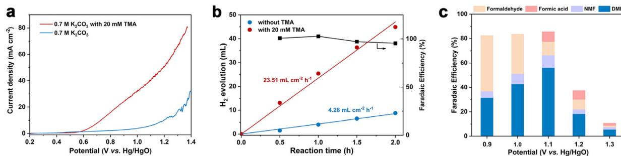
**Fig. 1** (a) LSV curves of a graphite flake at a scan rate of  $5 \text{ mV s}^{-1}$  in  $0.7 \text{ M K}_2\text{CO}_3$  with or without  $20 \text{ mM TMA}$ . (b)  $\text{H}_2$  production rate and faradaic efficiency at the cathode at  $1.1 \text{ V vs. Hg/HgO}$  in  $0.7 \text{ M K}_2\text{CO}_3$  with or without  $20 \text{ mM TMA}$ . (c) Faradaic efficiency as a function of applied potential for TMA oxidation.
