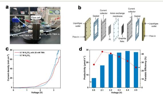
Fig. 3 Reaction evaluation in the MEA flow reactor. (a) Photograph of the MEA flow reactor. (b) Schematic illustration of the MEA flow reactor. (c) LSV curves at a scan rate of 10 mV s<sup>-1</sup> in 0.7 M K<sub>2</sub>CO<sub>3</sub> with or without 20 mM TMA at a flow rate of 5.4 mL min<sup>-1</sup>. (d) Productivity and faradaic efficiency as a function of potential. Reaction conditions:  $0.7 \text{ M K}_2\text{CO}_3$  with 20 mM TMA at a flow rate of  $5.4 \text{ mL min}^{-1}$ .
