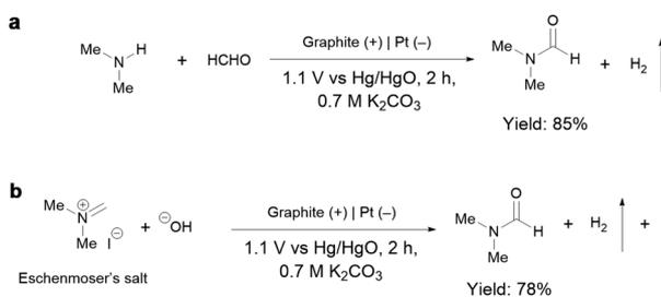
**Scheme 2** (a) Electrochemical oxidation of DMA and formaldehyde at 1.1 V vs. Hg/HgO under the standard conditions. (b) Electrochemical oxidation of Eschenmoser's salt at 1.1 V vs. Hg/HgO under the standard conditions.
