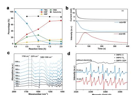
Fig. 2 (a) Time-dependent conversions of TMA in 0.7 M  $K_2CO_3$ . (b) DEMS results at 1.1 V vs. Hg/HgO in 0.7 M  $K_2CO_3$  with 20 mM TMA. (c) In situ IRRAS of the reaction in 0.7 M  $K_2CO_3$  with 20 mM TMA at 1.1 V vs. Hg/HgO. (d) EPR spectra of the reaction in 0.7 M  $K_2CO_3$  with 20 mM TMA at 1.1 V vs. Hg/HgO.
