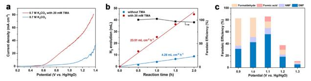
Fig. 1 (a) LSV curves of a graphite flake at a scan rate of 5 mV s<sup>-1</sup> in 0.7 M  $K_2CO_3$  with or without 20 mM TMA. (b)  $H_2$  production rate and faradaic efficiency at the cathode at 1.1 V vs. Hg/HgO in 0.7 M  $K_2CO_3$  with or without 20 mM TMA. (c) Faradaic efficiency as a function of applied potential for TMA oxidation.
