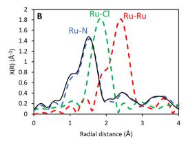
Fig. 3 XANES (A) and EXAFS (B) data for CBV-100-Ru(bipy)<sub>3</sub> (solid black) in comparison with reference samples (dashed lines): Ru(bipy)<sub>3</sub><sup>2+</sup>@EMC-1,<sup>27</sup> blue; RuCl<sub>3</sub>, green; Ru-foil, red.
