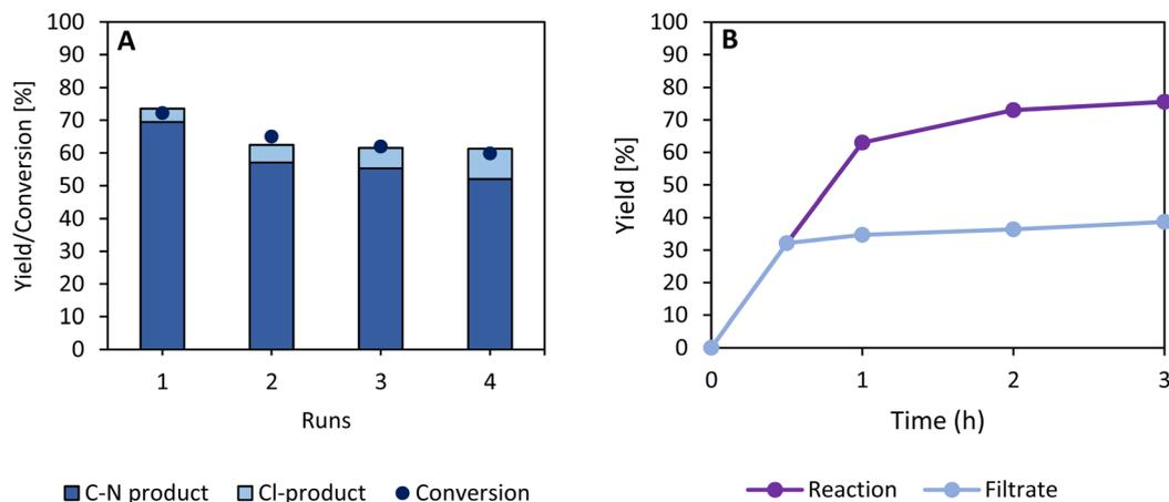
**Fig. 9** Recyclability test for four consecutive runs. A small reduction in yield was observed after four runs (A). After the reaction, the mixture was centrifuged, the reaction solution was removed and the zeolite was washed with ultrapure water and dried. Subsequently, fresh reaction mixture was added to the zeolite and a second/third/fourth run was executed. Filtration test was performed and filtrate was collected after 30 minutes to check the heterogeneity of the reaction (B).
