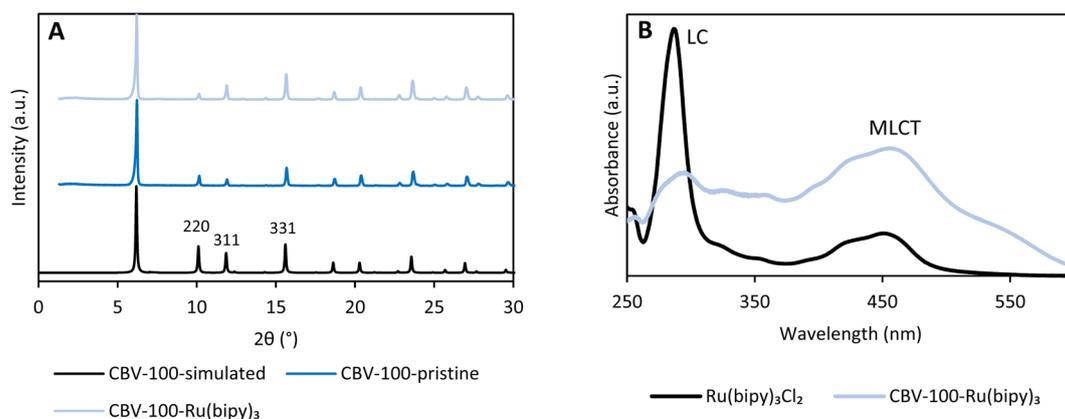
**Fig. 2** XRD diffractogram of simulated CBV-100 (black), pristine CBV-100 (dark blue) and Ru loaded CBV-100-Ru(bipy)<sub>3</sub> (light blue) (A). UV-Vis spectrum of the homogeneous complex in acetonitrile (Ru(bipy)<sub>3</sub>Cl<sub>2</sub>, black) and a diffuse reflectance spectrum of CBV-100-Ru(bipy)<sub>3</sub> (blue) (B). LC = ligand centered transition, MLCT = metal-to-ligand charge transfer.
