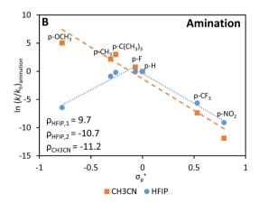
Fig. 5 Hammett plots of the homogeneous chlorination (A) and amination (B) reaction in HFIP and CH<sub>3</sub>CN. Only the product with the Cl<sup>-</sup> or amino-substituent on the para position is considered in these plots. Reaction conditions: 0.1 mmol piperidine, 1 equiv. NCS, 18 equiv. arene, 4 equiv. HClO<sub>4</sub>, 1 mL HFIP or CH<sub>3</sub>CN, 2 mol% Ru(bipy)<sub>3</sub>Cl<sub>2</sub>, 15 min, R.T.
