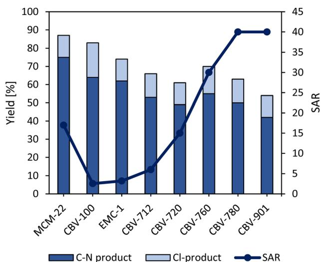
**Fig. 4** Product yields (dark blue line) for Ru(bpy)<sub>3</sub><sup>2+</sup> immobilized on zeolite supports with different SAR ratios (MCM-22 (SAR = 17), EMC-1 (SAR = 3.6), CBV-100 (SAR = 2.55), CBV-712 (SAR = 6), CBV-720 (SAR = 15), CBV-760 (SAR = 30), CBV-780 (SAR = 40) and CBV-901 (SAR = 40)). Reaction conditions: 0.1 mmol piperidine, 1 equiv. NCS, 18 equiv. *t*-butylbenzene, 4 equiv. HClO<sub>4</sub>, 1 mL HFIP, 2 mol% Ru as zeolite-Ru (theoretically), blue LEDs 3 h, R.T.
