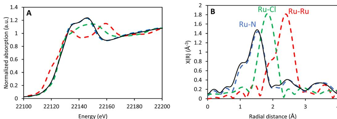
**Fig. 3** XANES (A) and EXAFS (B) data for CBV-100-Ru(bipy)<sub>3</sub> (solid black) in comparison with reference samples (dashed lines): Ru(bipy)<sub>3</sub><sup>2+</sup>@EMC-1,<sup>27</sup> blue; RuCl<sub>3</sub>, green; Ru-foil, red.
