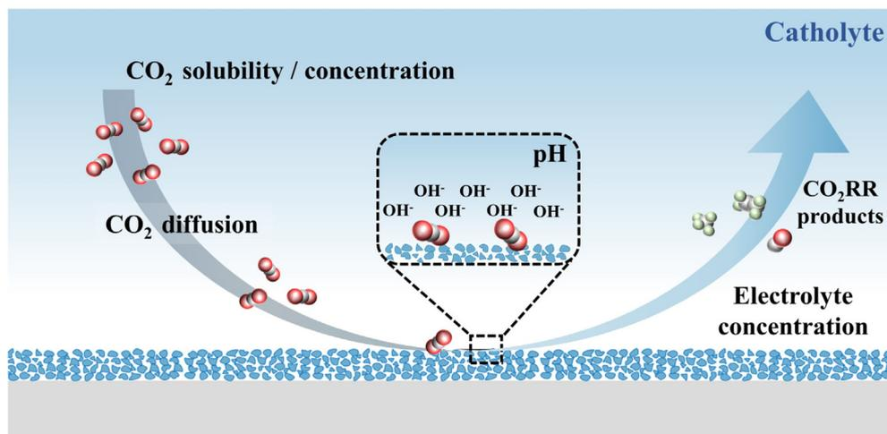
**Fig. 2** The influence factors of CO<sub>2</sub>RR performance, such as CO<sub>2</sub> solubility, CO<sub>2</sub> concentration, CO<sub>2</sub> diffusion coefficient, pH values and electrolyte concentration.
