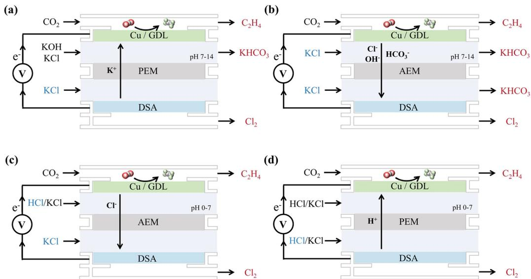
**Fig. 9** Four typical cell configurations of the CO<sub>2</sub>RR and Chlor-alkali reaction coupling system. The products are marked with a red color and the reactants that need to be supplemented are marked in blue color. (a) Cathodic alkaline environment with PEM; (b) Cathodic alkaline environment with AEM; (c) Cathodic acidic environment with AEM; (d) Cathodic acidic environment with PEM.
