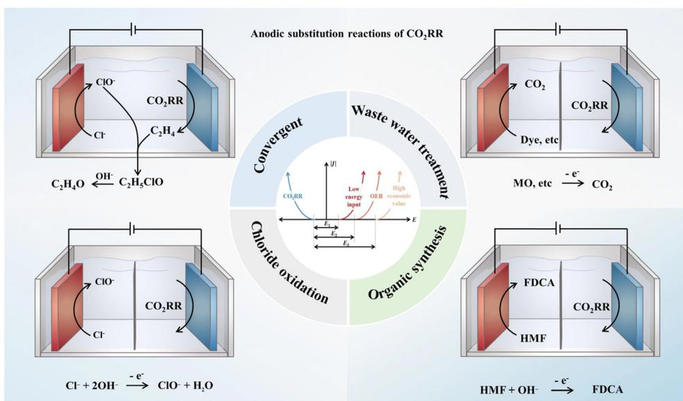
Fig. 1 Four typical types of alternative anode reactions of the CO<sub>2</sub>RR coupled system.
