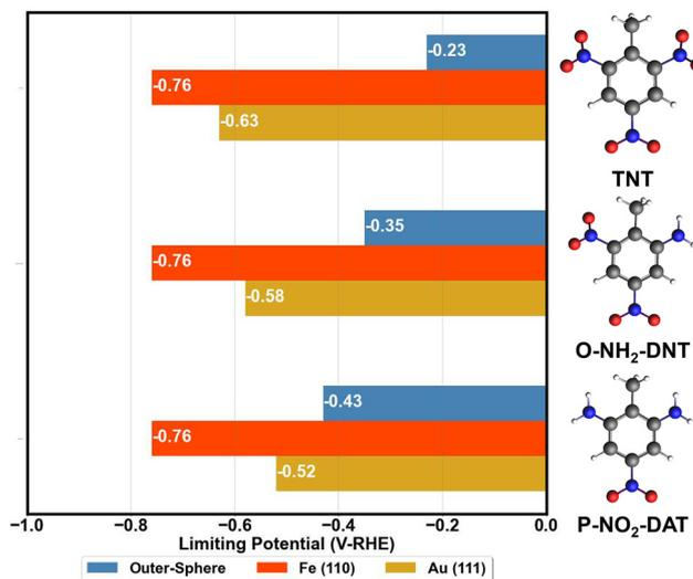
**Fig. 6** Comparison of DFT predicted TNT limiting potentials for outer-sphere and inner-sphere reduction. Limiting potentials are computed for the reduction of TNT to O-NH<sub>2</sub>-DNT then to P-NO<sub>2</sub>-DAT. Outer-sphere limiting potentials are calculated in G16/B3LYP/IEFPCM for coupled proton–electron transfer to reduce each NO<sub>2</sub> group. All reduction potentials are referred to the RHE scale. Atom colors are as follow: C = grey, N = blue, O = red, H = white.
