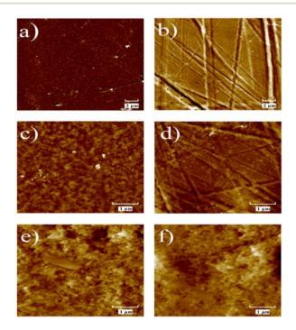
Fig. 1 Surface morphology of plastics substrate and graphite-coated screen-printed electrodes. Representative 20  $\mu$ m  $\times$  20  $\mu$ m AFM images: (a) Autostat<sup>TM</sup> polyester z scale = 100 nm; (b) post-consumer PET, z scale = 100 nm. Representative 5  $\mu$ m  $\times$  5  $\mu$ m AFM images: (c) Autostat<sup>TM</sup> polyester, z scale = 80 nm; (d) post-consumer PET, z scale = 50 nm; (e) SPE, z scale = 300 nm; (f) PET-SPE, z scale = 500 nm.
