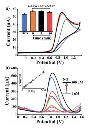
Fig. 5 Analytical performances of Bio-PET\_SPE based NO $_2^-$  sensor at different nitrite concentrations from 0 to 500  $\mu$ M in 0.01 M PBS (pH 7.4) by performing CV (a) and SWV (b) as electrochemical techniques. In the inset of Fig. (a) biochar's sorption effect on the analyte as a function of time is reported.
