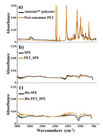
Fig. 2 ATR-FTIR characterization: (a) Autostat™ polyester and post-consumer PET, (b) Autostat™ polyester electrode (SPE) and post-consumer PET electrode (PET\_SPE), (c) biochar-modified electrodes: bio-SPE and Bio-PET\_SPE. Spectra are reported separately for clarity.
