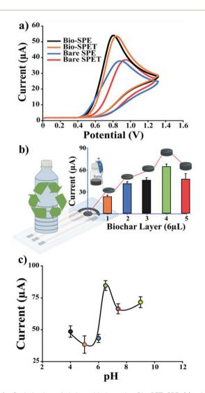
Fig. 4 Optimization of nitrite oxidation using Bio-PET\_SPE: (a) voltammograms obtained analysing a constant concentration of  $NO_2^-$  (100  $\mu$ M) using SPEs, PET-SPE, Bio-SPE and Bio-PET\_SPE; (b) SWV current as a function of the number of Biochar layers deposited at constant nitrite concentration; (c) currents as a function of pH.
