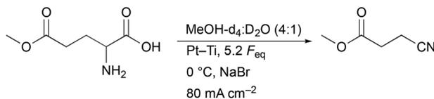
**Scheme 2** Conditions of the first experiment on the electro-oxidative decarboxylation of L-glutamic acid 5-methyl ester to CME. The concentration of L-glutamic acid 5-methyl ester was 0.2 M and the concentration of NaBr was 0.3 M. The studies of Dai *et al.* served as the basis for designing this experiment.<sup>15</sup>
