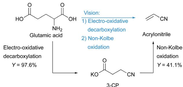
**Scheme 5** Vision for the synthesis of acrylonitrile using electro-oxidative decarboxylation and non-Kolbe electrolysis (light blue). So far, the one-pot synthesis has not been realised. However, it was shown that in principle acrylonitrile can be produced from glutamic acid using electrochemistry.
