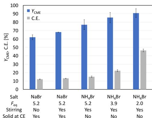
**Fig. 1** Variation of the reaction conditions and their influence on yield ( $Y_{\text{CME}}$ ) and current efficiency (C.E.) for the synthesis of CME. Conditions: Pt-Ti; solvent: MeOH- $d_4$ :  $\text{D}_2\text{O}$  (4 : 1); L-glutamic acid 5-methyl ester: 0.2 M (1 eq.); mediator salt: 0.3 M (1.5 eq.);  $j = 80 \text{ mA cm}^{-2}$ ; and  $T = 0 \text{ }^\circ\text{C}$ .
