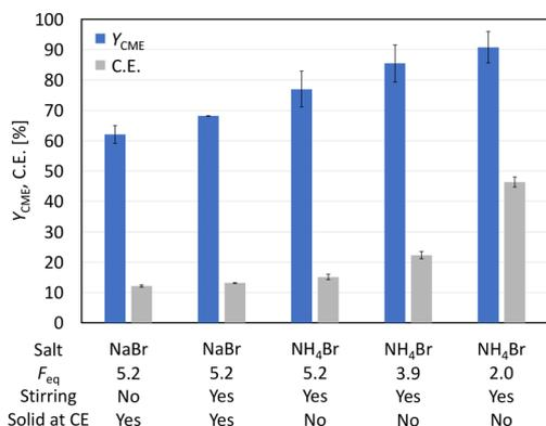
**Fig. 1** Variation of the reaction conditions and their influence on yield ( $Y_{\text{CME}}$ ) and current efficiency (C.E.) for the synthesis of CME. Conditions: Pt-Ti; solvent:  $\text{MeOH-d}_4 : \text{D}_2\text{O}$  (4 : 1); L-glutamic acid 5-methyl ester: 0.2 M (1 eq.); mediator salt: 0.3 M (1.5 eq.);  $j = 80 \text{ mA cm}^{-2}$ ; and  $T = 0 \text{ }^\circ\text{C}$ .
