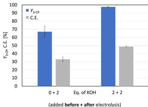
**Fig. 2** Electro-oxidative decarboxylation of D,L-glutamic acid to 3-CP. Investigating the impact of the addition of 0 eq. or 2 eq. of KOH to the substrate solution on the yield of 3-CP and the current efficiency. Conditions: Pt-Ti; solvent: D<sub>2</sub>O; D,L-glutamic acid: 0.2 M (1 eq.); NH<sub>4</sub>Br: 0.3 M (1.5 eq.); KOH (after electrolysis): 2 eq.;  $F_{eq} = 2.0$ ;  $j = 80 \text{ mA cm}^{-2}$ ; and  $T = 0 \text{ }^\circ\text{C}$ .
