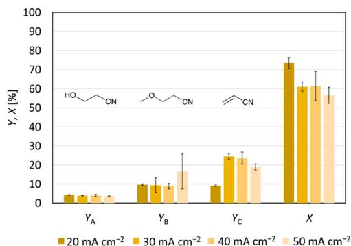
**Fig. 3** Effects of the current density on the yield of acrylonitrile ( $Y_C$ ) and the two Hofer–Moest side products 3-hydroxypropanenitrile ( $Y_A$ ) and 3-methoxypropanenitrile ( $Y_B$ ). Furthermore, the conversion of the substrate ( $X$ ) is visualised. Conditions: C<sub>gr</sub>-Ti; solvent: MeOH-d<sub>4</sub>; 3-CP: 0.071 M;  $F_{eq} = 1.0$ ; stirring; and  $T = 0 \text{ }^\circ\text{C}$ .
