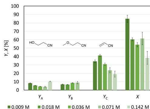
**Fig. 5** Effects of the initial 3-CP concentration on the yield of acrylonitrile ( $Y_C$ ) and the two Hofer–Moest side products 3-hydroxypropanenitrile ( $Y_A$ ) and 3-methoxypropanenitrile ( $Y_B$ ). Furthermore, the conversion of the substrate ( $X$ ) is visualised. Conditions:  $C_{\text{gr-Ti}}$ ; solvent: MeOH- $d_4$ ;  $F_{\text{eq}} = 1.0$ ;  $j = 40 \text{ mA cm}^{-2}$ ; stirring; and  $T = 0 \text{ }^\circ\text{C}$ .
