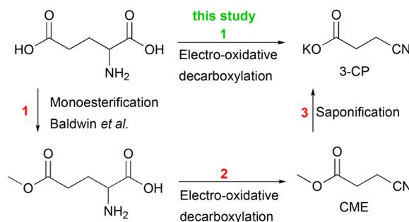
**Scheme 3** The current pathway from  $D,L$ -glutamic acid to 3-CP requires 3 steps (red) and thus is neither step-efficient nor atom-efficient.<sup>15</sup> The synthesis of 3-CP can be more sustainable if  $D,L$ -glutamic acid is decarboxylated without pre-modification (green, this study).
