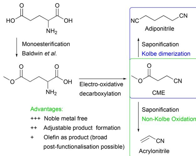
**Scheme 1** An environmentally friendly pathway to produce adiponitrile from glutamic acid *via* 3 steps according to Dai *et al.* (blue box)<sup>15</sup> and applying non-Kolbe conditions to potassium 3-cyanopropanoate (3-CP), obtained by saponification of 3-cyanopropanoic acid methyl ester (CME) by KOH to synthesise acrylonitrile (green box).
