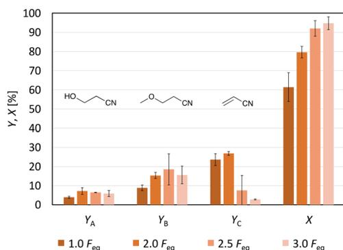
**Fig. 4** Effects of the Faraday equivalents on the yield of acrylonitrile ( $Y_C$ ) and the two Hofer–Moest side products 3-hydroxypropanenitrile ( $Y_A$ ) and 3-methoxypropanenitrile ( $Y_B$ ). Furthermore, the conversion of the substrate ( $X$ ) is visualised. Conditions:  $C_{\text{gr-Ti}}$ ; solvent: MeOH- $d_4$ ; 3-CP: 0.071 M;  $j = 40 \text{ mA cm}^{-2}$ ; stirring; and  $T = 0 \text{ }^\circ\text{C}$ .
