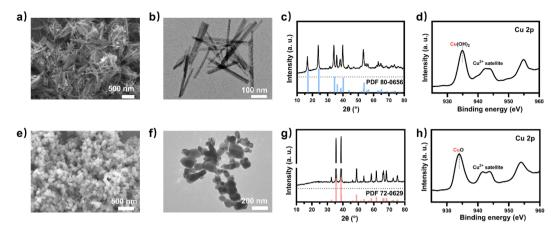
Fig. 3 (a) SEM image and (b) TEM image of Cu(OH)<sub>2</sub>. (c) XRD revealed peaks assignable to the pattern of Cu(OH)<sub>2</sub> (reference peaks from JCPDS Data Card No. 80-0656 given as drop lines). (d) XPS spectra of Cu 2p for Cu(OH)2. (e) SEM image and (f) TEM image of the model electrocatalyst CuO. (g) XRD revealed peaks assignable to the pattern of CuO (reference peaks from JCPDS Data Card No. 72-0629 given as drop lines). (h) XPS spectra of Cu 2p for CuO.
