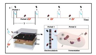
Scheme 1 Schematic illustration of an electro-bio tandem reactor assembled with copper nanoparticles and microbes. In one cycle time (T), copper was used as the model electrocatalyst to reduce CO<sub>2</sub> to multicarbon products (ethylene) in a flow cell (Period 1). Then, Moorella thermoacetica metabolized the concomitant products such as HCOOH, CO, and  $H_2$  to acetate through the Wood-Ljungdahl pathway (Period 2).
