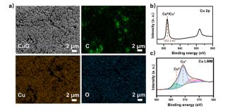
Fig. 5 The GDL cathode loaded with the nano-Cu catalyst was analyzed after the tandem experiment. (a) SEM image and EDX maps of the catalyst on GDL showed uniform Cu and O distribution. All scale bars are 2  $\mu$ m. (b) Cu 2p XPS spectra and (c) Cu LMM Auger spectra of the nano-Cu catalyst.
