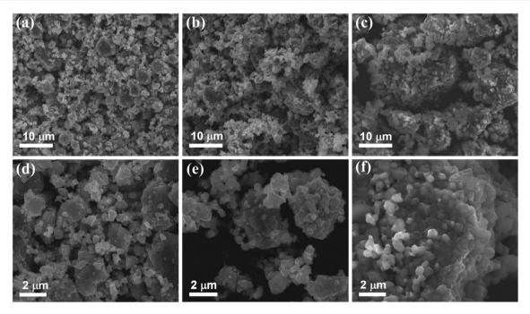
Fig. 4 SEM images at low and high magnifications for ball-milled ( $Li_2Fe$ )SO (a and d) and ball-milled ( $Li_2Fe$ )SO followed by post-heat treating at 300 °C (b and e) and 500 °C (c and f).
