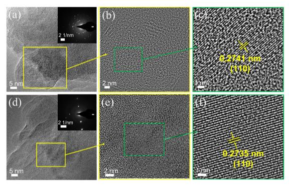
Fig. 5 TEM images for ball-milled ( $\text{Li}_2\text{Fe}$ )SO (a-c) and ball-milled ( $\text{Li}_2\text{Fe}$ )SO followed by post-heat treatment at 500 °C (d-f). The insets in Fig. 5a and d present the SEAD images.
