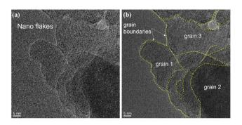
Fig. 6 TEM image without (a) and with (b) marking the grain boundaries (yellow dashed lines) between the agglomerated grains/flakes of ball-milled (Li<sub>2</sub>Fe)SO.
