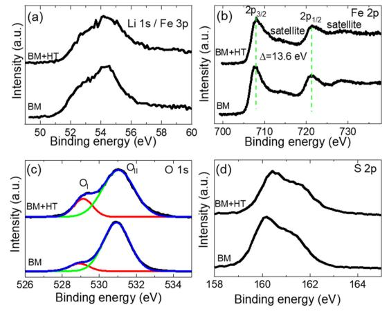
Fig. 8 XPS high-resolution spectrum of (a) Li 1s/Fe 3p, (b) Fe 2p, (c) O 1s, and (d) S 2p for (Li<sub>2</sub>Fe)SO prepared by direct ball-milling (BM) and ball-milling followed by post-heat treatment at 500 °C (BM + HT).
