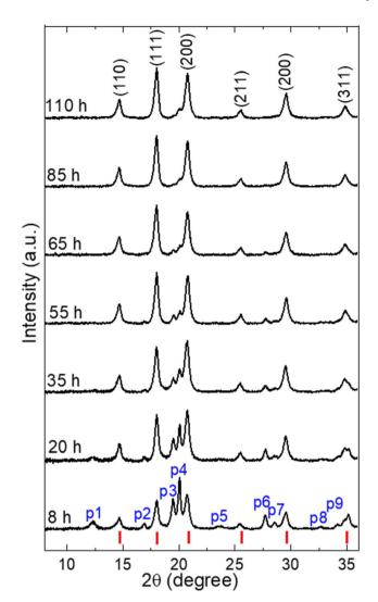
Fig. 2 XRD patterns of the milled powder as a function of the milling time using 3:1 as BPR. The labels (p1-p9) refer to the secondary phases, while the red marks (as reference) refer to the ideal Bragg positions of (Li<sub>2</sub>Fe)SO.
