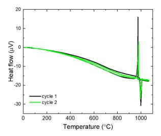
Fig. 7 DTA for ball-milled (Li<sub>2</sub>Fe)SO.
