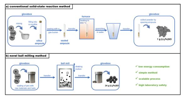
Fig. 1 Schematic diagram of the synthesis procedures of (Li<sub>2</sub>Fe)SO by the reported solid state reaction (a) and the novel mechanochemical (b) methods.
