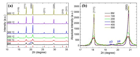
Fig. 3 Influence of the heat treatment temperature on the XRD of ball-milled (Li<sub>2</sub>Fe)SO (BM) (a) and on the XRD intensity of (111) and (200) peaks (b). The red marks in (a) refer to the ideal Bragg positions of (Li<sub>2</sub>Fe)SO as a reference.
