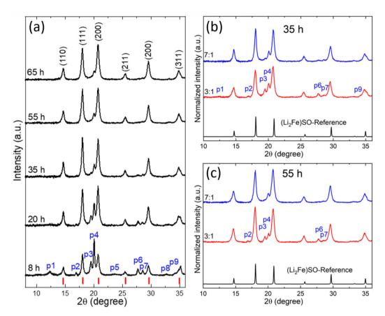
Fig. 9 XRD patterns of the milled powder as a function of the milling time using 7:1 as BPR (a) and comparison between different BPRs (3:1 and 7:1) at two milling times (b and c). The labels (p1-p9) refer to the secondary phases, while the red short lines in (a) represent the ideal Bragg positions for the ( $Li_2Fe$ )SO phase.
