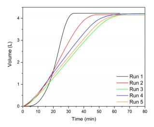
Fig. 5 Cumulative  $H_2$  volume generated in the presence of cobalt chitosan spheres over multiple runs. 5  $\times$  50 mL volume runs were done back-to-back with no drying of the catalyst in between. Measurements were recorded using mass flow meters every second (see Experimental section for details).
