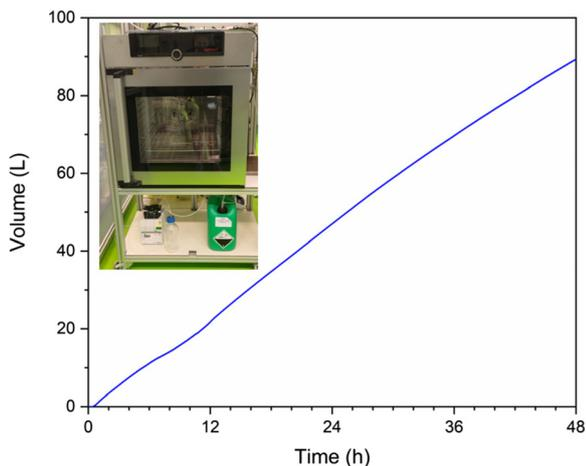
**Fig. 7** Cumulative  $H_2$  volume generated in continuous reactor by cobalt chitosan spheres over a 48 h period. Measurements taken once per second using mass flow meters. The inset shows a photo of the system with the fuel vat, pump, reactor oven and waste vat. A detailed description of the reactor system is included in the ESI.†
