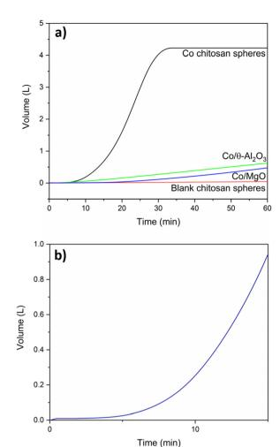
Fig. 4 Cumulative  $H_2$  volume of cobalt chitosan spheres v blank chitosan spheres (a) and cobalt chitosan sphere activation period (b). Measurements were recorded using mass flow meters every second (see Experimental section for details).
