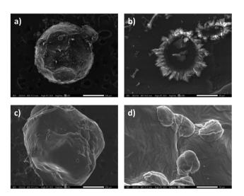
Fig. 2 SEM images of the surface of a cobalt chitosan sphere with  $50 \times$  (a) and  $500 \times$  magnification (b). SEM images of blank (metal-free) chitosan spheres at  $50 \times$  magnification (c) and  $500 \times$  magnification (d). All images are of pristine catalysts.
