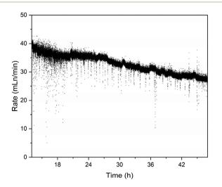
Fig. 8 Rate of H<sub>2</sub> generation measured by mass flow meters in a continuous reactor (measurements taken once per second).
