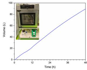
Fig. 7 Cumulative  $H_2$  volume generated in continuous reactor by cobalt chitosan spheres over a 48 h period. Measurements taken once per second using mass flow meters. The inset shows a photo of the system with the fuel vat, pump, reactor oven and waste vat. A detailed description of the reactor system is included in the ESI.†
