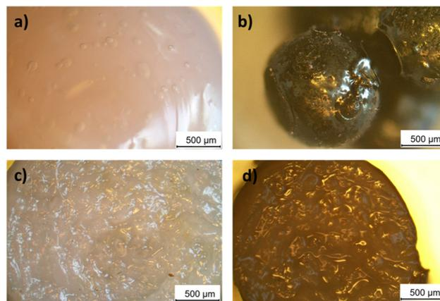
Fig. 1 Optical microscopy images of the surface of the cobalt gel and dried spheres (a and b) and cross-section the same gel and dried spheres (c and d) respectively. Images were taken at 50x magnification. All images are of pristine catalysts.
