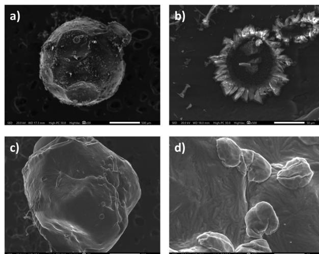
Fig. 2 SEM images of the surface of a cobalt chitosan sphere with 50x (a) and 500x magnification (b). SEM images of blank (metal-free) chitosan spheres at 50x magnification (c) and 500x magnification (d). All images are of pristine catalysts.
