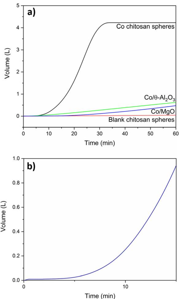
Fig. 4 Cumulative  $H_2$  volume of cobalt chitosan spheres v blank chitosan spheres (a) and cobalt chitosan sphere activation period (b). Measurements were recorded using mass flow meters every second (see Experimental section for details).
