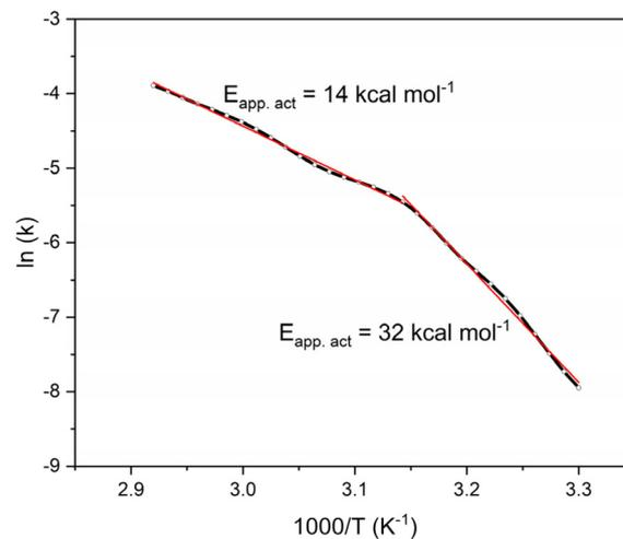
**Fig. 6** Arrhenius plot for the catalytic hydrolysis of  $\text{KBH}_4$  using a single cobalt chitosan sphere. The experiment was done using a high precision bubble counter in triplicate (see Experimental section for details). The graph is based on 300 data points, of which only 30 are shown for clarity.
