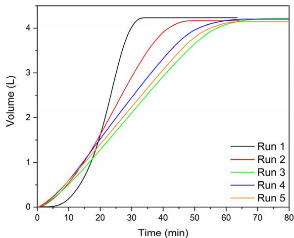
**Fig. 5** Cumulative  $\text{H}_2$  volume generated in the presence of cobalt chitosan spheres over multiple runs.  $5 \times 50$  mL volume runs were done back-to-back with no drying of the catalyst in between. Measurements were recorded using mass flow meters every second (see Experimental section for details).
