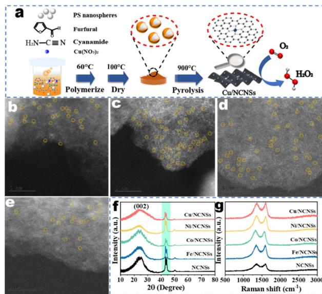
**Fig. 1** The synthetic process of M/NCNSs (a), high-resolution HAADF-STEM images of Fe/NCNSs (b), Co/NCNSs (c), Ni/NCNSs (d), and Cu/NCNSs (e), XRD patterns (f) and Raman spectra (g) of the as-synthesized samples.
