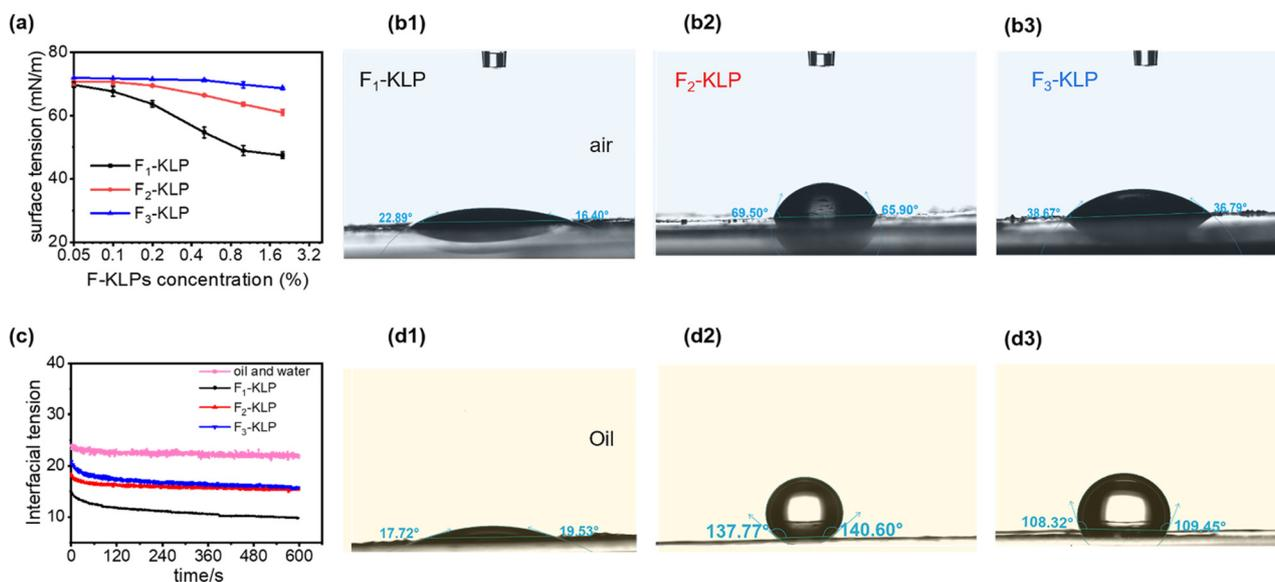
Fig. 4 Wettability of  $F_n$ -KLP at the air/water and oil/water interfaces. (a) Surface tension as a function of  $F_n$ -KLP concentration. (b1–b3) Water contact angles of  $F_n$ -KLP. (c) Changes in interfacial tension as a function of time, and (d1–d3) three-phase contact angles for  $F_n$ -KLP between sunflower oil and water.
