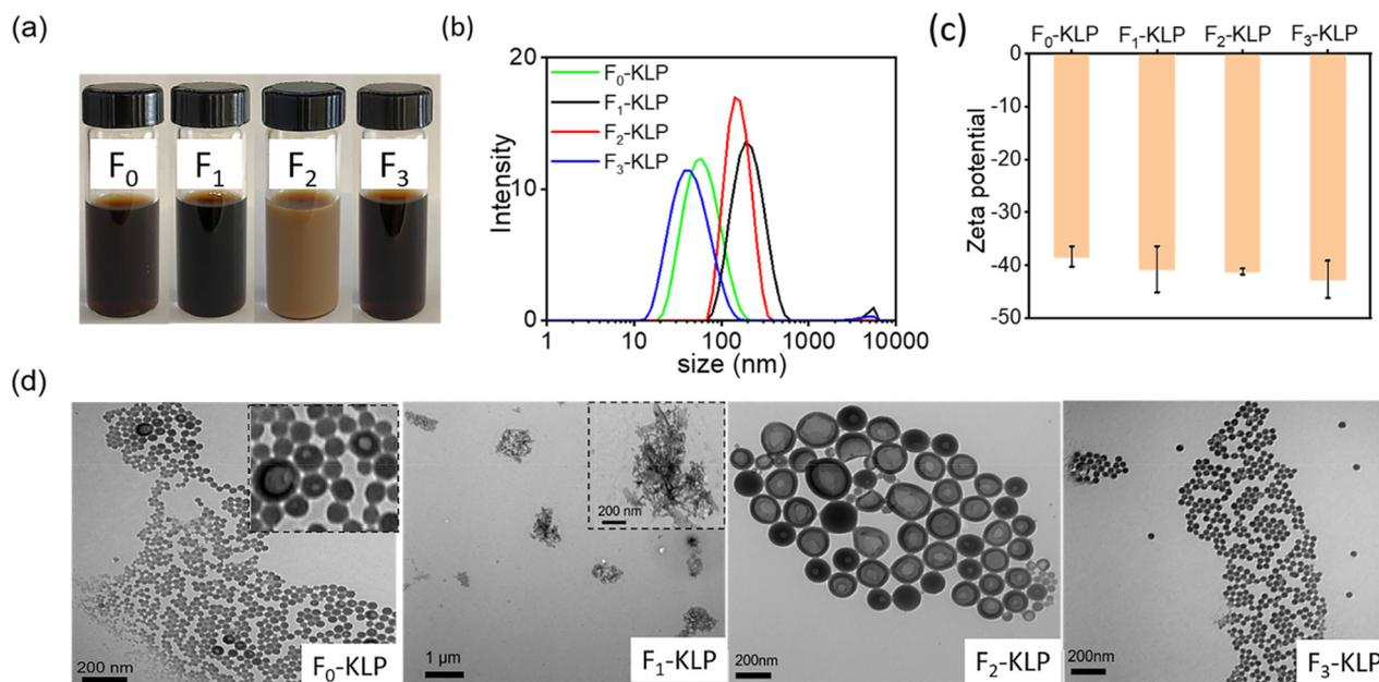
Fig. 3  $F_n$ -KLP colloidal characteristics: (a) digital photographs of the colloidal suspensions of  $F_n$ -KLP (0.5%), (b) size distribution, (c)  $\zeta$ -potential and (d) TEM images of  $F_n$ -KLP.
