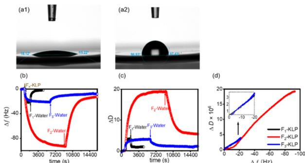
**Fig. 6** Contact angles of water on (a1) a gold-coated QCM sensor and (a2) a sensor coated with sunflower oil. Changes of  $\Delta f$  (b) and  $\Delta D$  (c) with time during the adsorption and desorption of  $F_n$ -KLP on a quartz crystal sensor coated with sunflower oil. (d)  $\Delta D$ - $\Delta f$  plots describing the particle adsorption process.
