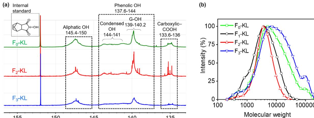
Fig. 2 Chemical characterization of  $F_n$ -KL: (a)  $^{31}\text{P}$ -NMR spectra and (b) molecular weight distribution (GPC).
