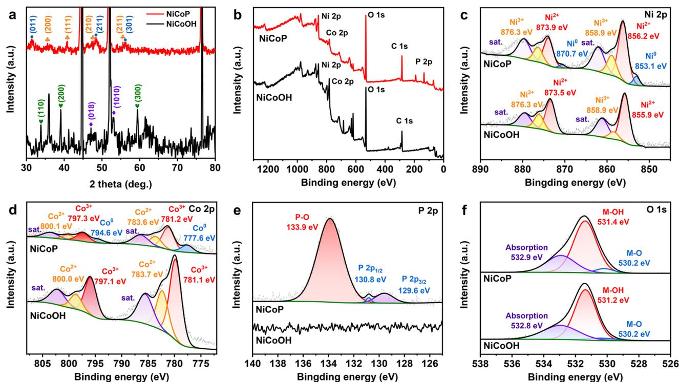
Fig. 2 (a) XRD patterns and XPS spectra of (b) broad scans, (c) Ni 2p, (d) Co 2p, (e) P 2p and (f) O 1s of NiCoP and NiCoOH electrocatalysts.
