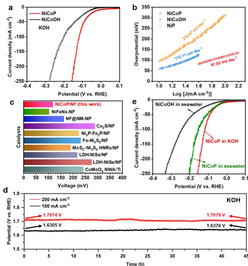
**Fig. 4** (a) LSV curves and (b) the corresponding Tafel plots of NiCoOH and NiCoP electrocatalysts in 1.0 M KOH. (c) A comparison of the HER in 1.0 M KOH at a current density of 100 mA cm<sup>-2</sup> between NiCoP and other noble-metal catalysts reported to date. (d) 45 h stability test of NiCoP for a cathodic HER at 100 and 200 mA cm<sup>-2</sup> and (e) LSV curves of the NiCoOH and NiCoP electrocatalysts in 1.0 M KOH and alkaline seawater.
