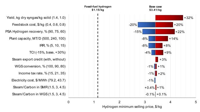
Fig. 6 Sensitivity analysis for the MPW-hydrogen process. The largest impact on MSP is from syngas yield (kg dry syngas per kg solid feedstock) and waste plastic feedstock cost (\$0.60 kg<sup>-1</sup>). Discussion on syngas yield is included in the caption of Fig. 3. Sensitivity analysis for the MSW-hydrogen process is shown in Fig. S8.†
