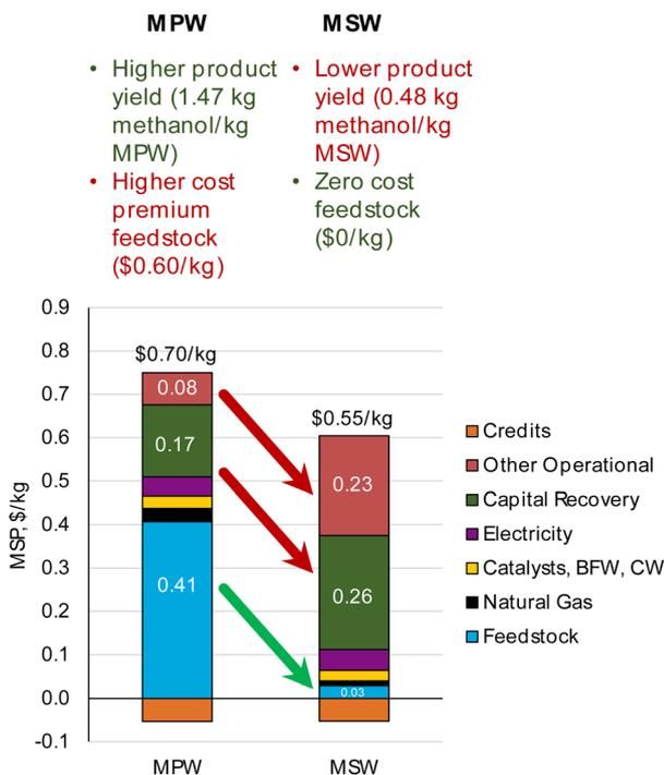
**Fig. 10** Comparison of MSP breakdown of methanol obtained from MPW and MSW gasification. Comparing MPW and MSW, the large reduction of feedstock contribution to MSP in MSW is accompanied by a simultaneous increase in the capital cost and other operational costs (fixed cost) due to the lower product yield of the MSW-methanol process.
