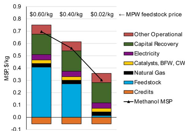
Fig. 9 Methanol MSP for varied MPW feedstock prices. Cost parity with fossil-fuel-based methanol (\$0.30 kg<sup>-1</sup>) could be achieved if MPW feedstock is available for ≤\$0.02 kg<sup>-1</sup>.
