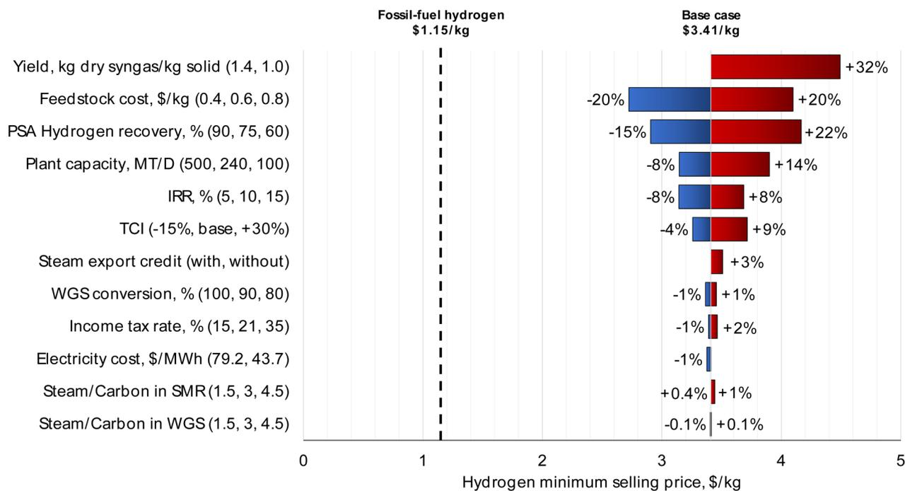
**Fig. 6** Sensitivity analysis for the MPW-hydrogen process. The largest impact on MSP is from syngas yield (kg dry syngas per kg solid feedstock) and waste plastic feedstock cost ( $\$0.60 \text{ kg}^{-1}$ ). Discussion on syngas yield is included in the caption of Fig. 3. Sensitivity analysis for the MSW-hydrogen process is shown in Fig. S8.†
