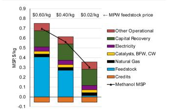
Fig. 9 Methanol MSP for varied MPW feedstock prices. Cost parity with fossil-fuel-based methanol ( $$0.30~{\rm kg}^{-1}$$ ) could be achieved if MPW feedstock is available for  $\le$  $$0.02~{\rm kg}^{-1}$ .
