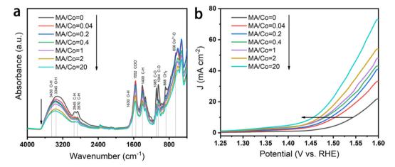
Fig. 4 Influence of the MA/Co molar ratio on the electrocatalytic performance of  $CoO_xH_{y\cdot}$  (a) FTIR spectra and (b) LSVs in 1 M KOH solution containing 10 mM HMF at a scanning rate of 10 mV s<sup>-1</sup>.
