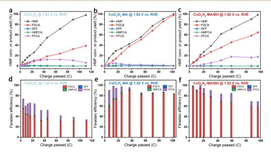
Fig. 5 Results of HMFOR using CoO<sub>x</sub>H<sub>v</sub>, CoO<sub>x</sub>H<sub>v</sub>-MA, and CoO<sub>x</sub>H<sub>v</sub>-MA/BH at a constant potential of 1.52 V vs. RHE in 1 M KOH containing 5 mM HMF, after passing various amounts of charges. (a, b and c) The conversion of HMF and the yields of oxidation products, and (d, e and f) the corresponding faradaic efficiencies of (a and d)  $CoO_xH_v$ , (b and e)  $CoO_xH_v$ -MA, and (c and f)  $CoO_xH_v$ -MA/BH, respectively.
