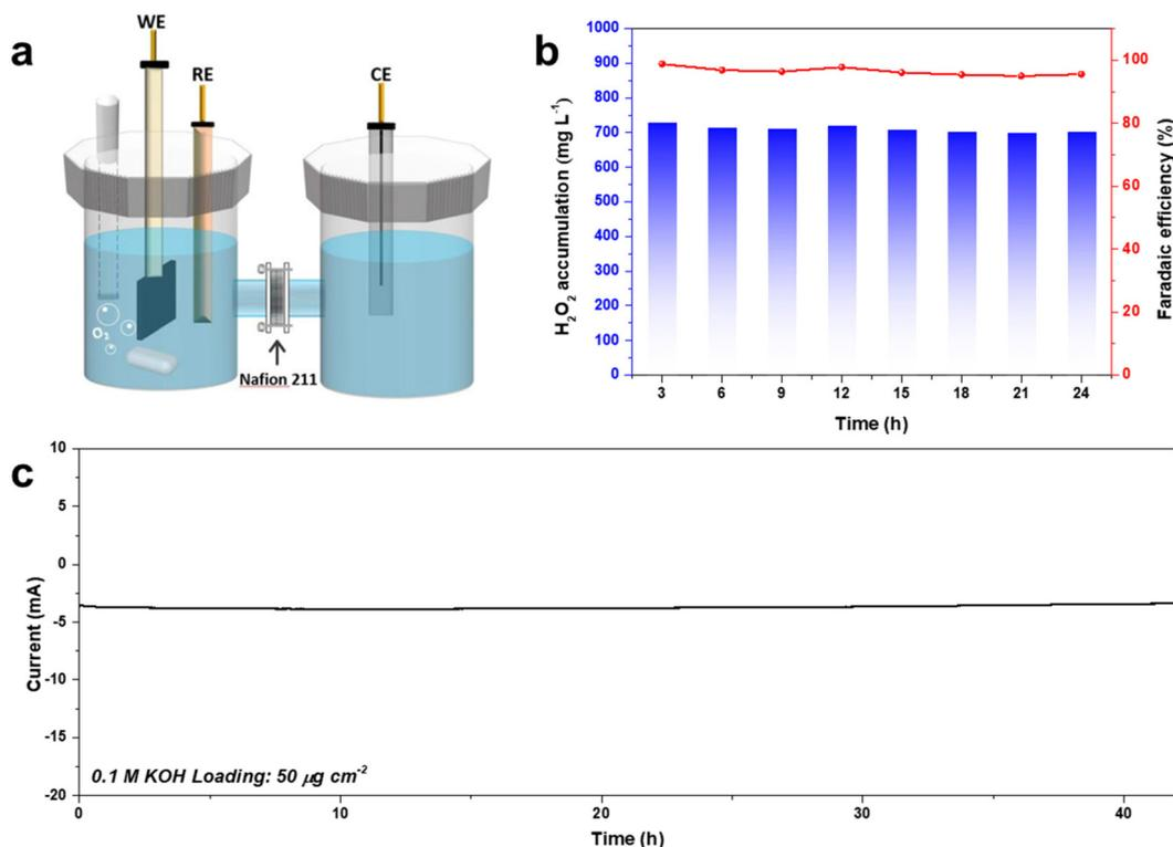
Fig. 8 (a) Schematic of the bulk H<sub>2</sub>O<sub>2</sub> production device. (b) The FE% and concentration of the produced H<sub>2</sub>O<sub>2</sub> using CA-NR. (c) Long-term stability test of CA-NR at 0.65 V.
