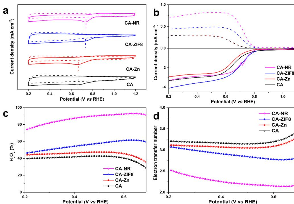
Fig. 6 (a) Cyclic voltammograms of samples in  $\text{O}_2$ -saturated 0.1 M KOH at  $10 \text{ mV s}^{-1}$ . (b) Polarization curves of samples at 1600 rpm in  $\text{O}_2$ -saturated 0.1 M KOH (dashed lines: ring current; solid lines: disk current). (c)  $\text{H}_2\text{O}_2$  selectivity of samples. (d) Electron transfer number of samples.
