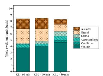
Fig. 8 Yields of phenolic compounds during KBL and KL catalytic oxidation. Operating conditions: 150 °C, 20 bar air, stirring 1800 rpm, 30-60 min, dry matter concentration 5 g L<sup>-1</sup>, copper/lignin mass ratio 5%
