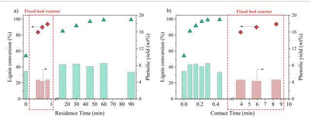
Fig. 11 Lignin conversion and phenolics production during KBL catalytic oxidation, represented as a function of residence time (a) or contact time (b). Operating conditions: 150 °C, 20-80 bar air, dry matter concentration 5 g L<sup>-1</sup>, catalyst CuO/TiO<sub>2</sub>.
