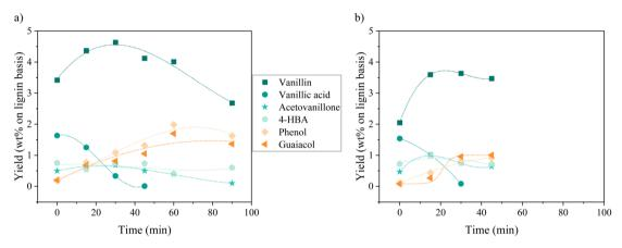
Fig. 2 Yields of phenolic compounds as a function of time during KBL oxidation for catalysed (a) and non-catalysed (b) reactions. Operating conditions: 150 °C, 20 bar air, stirring 1800 rpm, dry matter concentration 5 g L<sup>-1</sup>, copper/dry matter ratio 5%. Lines are only guides for the eyes. 4-HBA: 4-hydroxy-benzoic acid.
