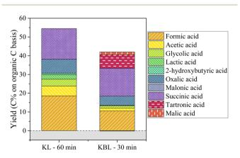
Fig. 9 Aliphatic compounds production after PL and KBL oxidation. Operating conditions: 150 °C, 20 bar air, stirring 1800 rpm, 30–60 min, dry matter concentration 5 g  $L^{-1}$ , copper/dry matter mass ratio 5%.
