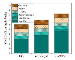
Fig. 4 Yields of phenolic compounds during KBL oxidation for non-catalysed and catalysed reactions. Operating conditions: 150 °C, 20 bar air, stirring 1800 rpm, dry matter concentration 5 g L<sup>-1</sup>, copper/dry matter mass ratio 5%, 30 min.
