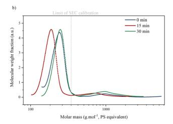
**Fig. 6** SEC analysis of Klason phases during catalytic (a) or non-catalytic (b) oxidation of KBL. Operating conditions: 150 °C, 20 bar air, stirring 1800 rpm, dry matter concentration 5 g L $^{-1}$ , copper/dry matter ratio 5%.
