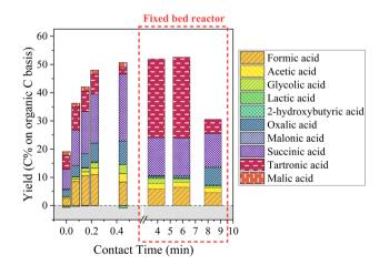
Fig. 13 Aliphatic compounds production during KBL catalytic oxidation. Operating conditions: 150 °C, 20-80 bar air, dry matter concentration 5 g L<sup>-1</sup>, catalyst CuO/TiO<sub>2</sub>.
