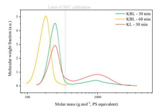
Fig. 10 SEC analysis of Klason phases during catalytic oxidation of KL or KBL. Operating conditions: 150 °C, 20 bar air, stirring 1800 rpm, dry matter concentration 5 g  $\rm L^{-1}$ , copper/dry matter ratio 5%.
