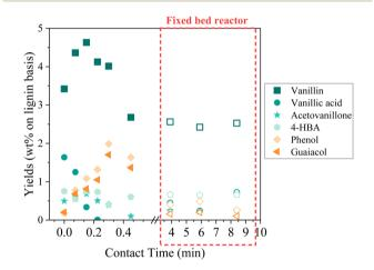
Fig. 12 Details of phenolics production during KBL catalytic oxidation. Operating conditions: 150 °C, 20-80 bar air, dry matter concentration 5 g L<sup>-1</sup>, catalyst CuO/TiO<sub>2</sub>.
