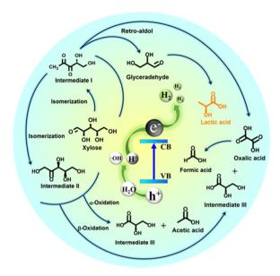
Fig. 8 Possible reaction mechanism of the photocatalytic co-production of hydrogen and lactic acid *via* RuS<sub>2</sub>@CN-2.
