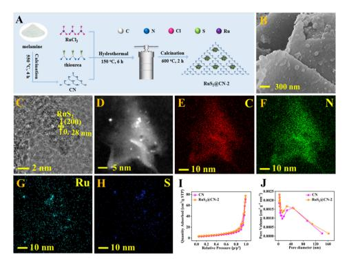
Fig. 1 Preparation scheme of RuS<sub>2</sub>@CN-x (A). SEM image (B) and TEM images (C and D) of RuS<sub>2</sub>@CN-2. Elemental mapping images of RuS<sub>2</sub>@CN-2: C (E), N (F), Ru (G), S (H). N<sub>2</sub> adsorption—desorption isotherms of CN and RuS<sub>2</sub>@CN-2 (J). Pore width distribution of CN and RuS<sub>2</sub>@CN-2 (J).
