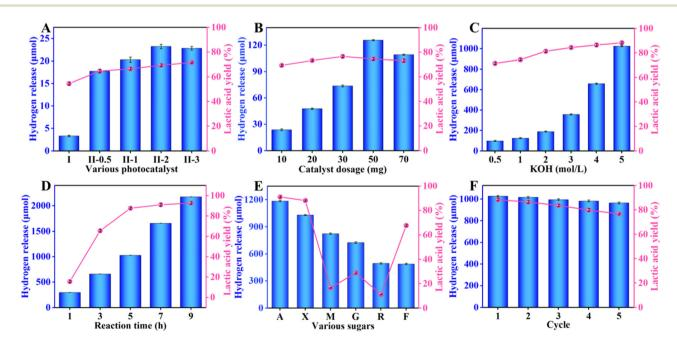
Fig. 4 The effects of various conditions on co-production of hydrogen and lactic acid, (A) different photocatalysts (I: CN, II: RuS<sub>2</sub>@CN), (B) catalyst dosages (5.0 h, 30 °C), (C) KOH concentrations (10.0 mg RuS<sub>2</sub>@CN-2, 5.0 h), (D) irradiation time (10 mg RuS<sub>2</sub>@CN-2, 5.0 M KOH). (E) The selective oxidation of different biomass-derived sugars to hydrogen and lactic acid photocatalyzed by RuS<sub>2</sub>@CN-2. (F) Recycling test of RuS<sub>2</sub>@CN-2.
