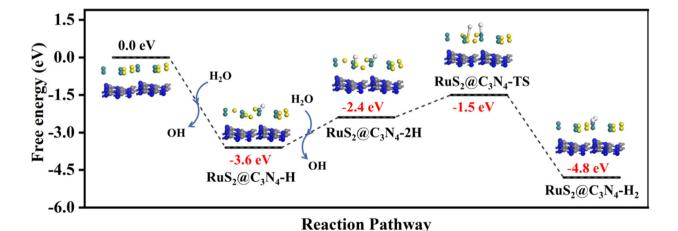
Fig. 7 The hydrogen generation pathway calculated by DFT.
