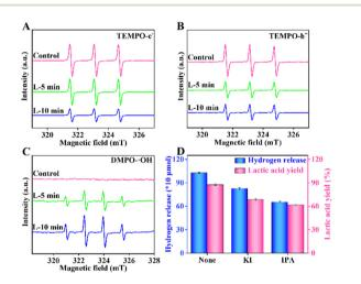
Fig. 6 TEMPO ESR spin-labelling for  $e^-$  (A) and  $h^+$  (B) of RuS<sub>2</sub>@CN-2. DMPO ESR spin-labelling for 'OH of RuS<sub>2</sub>@CN-2 (C). The effects of different oxidation active species on the photocatalytic performances (D).
