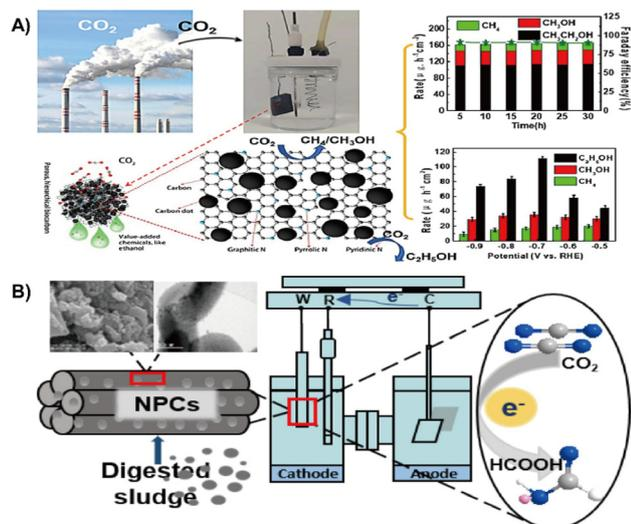
**Fig. 12** (A) Municipal sludge derived carbon dots modified, N-doped biochar for the electrochemical reduction of carbon dioxide.<sup>28</sup> Reprinted with permission. Copyright 2022, Elsevier. (B) Nitrogen-doped porous carbon from digested sludge for the electrochemical reduction of carbon dioxide to formate.<sup>135</sup> Reprinted with permission. Copyright 2018, American Chemical Society.
