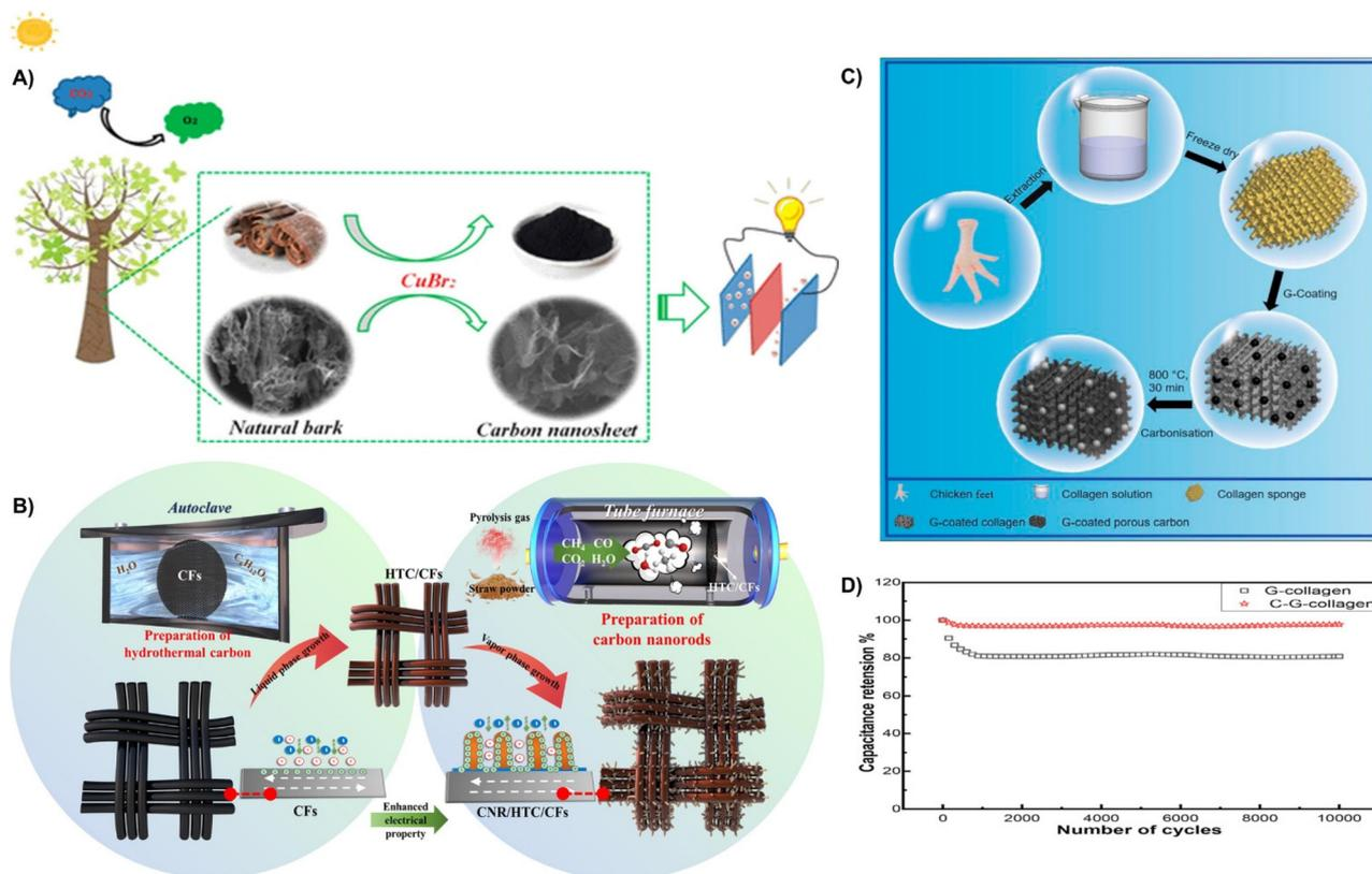
**Fig. 22** (A) Preparation of the 3D porous carbon nanosheet.<sup>220</sup> Reprinted with permission. Copyright 2019, American Chemical Society. (B) The schematic diagram of the synthesis of CNR/HTC/CFs.<sup>219</sup> Reprinted with permission. Copyright 2021, Elsevier. (C) Schematic demonstration of collagen, G-collagen, and C-G-collagen fabrication. (D) Cyclic study of C-G-collagen.<sup>223</sup> Reprinted with permission. Copyright 2022, Elsevier.
