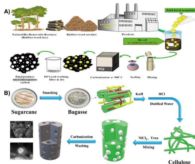
Fig. 19 (A) Schematic designs of resource collection and synthesis route of hierarchical porous hard carbon.<sup>197</sup> Reprinted with permission. Copyright 2019, Elsevier. (B) Flow chart of as-synthesized biomass porous carbon materials.<sup>201</sup> Reprinted with permission. Copyright 2021, Elsevier.
