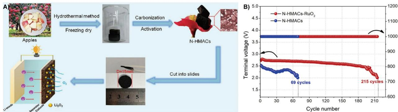
Fig. 18 (A) The synthesis strategy of N-HMACs and the construction of a Li- $\text{O}_2$  battery with an N-HMAC cathode. (B) Voltage of the terminal discharge and the cycle number.<sup>195</sup> Reprinted with permission. Copyright 2020, Elsevier.
