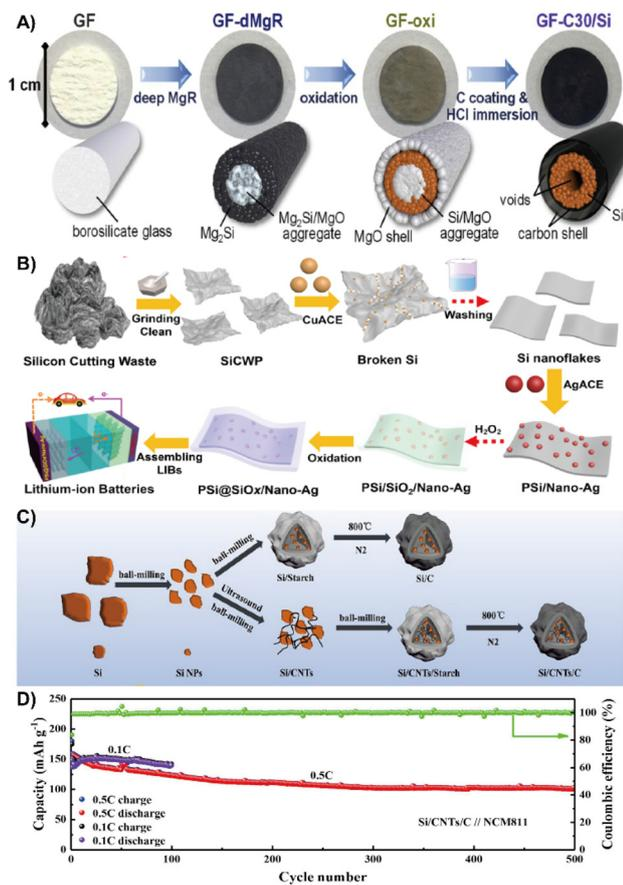
**Fig. 15** (A) Preparation process diagram of the GF-C30/Si suspended electrode.<sup>164</sup> Reprinted with permission. Copyright 2020, Elsevier. (B) Fabrication of the Si@SiO<sub>x</sub>/Nano-Ag composite.<sup>32</sup> Reprinted with permission. Copyright 2021, Elsevier. (C) An overall illustration of a typical recovery and conversion process. (D) Long-term cycling performance at 0.5 C.<sup>167</sup> Reprinted with permission. Copyright 2022, Elsevier.
