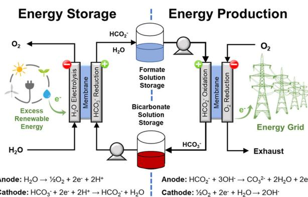
Fig. 8 Conceptual depiction of the electrochemical formate-bicarbonate cycle to store and to release energy. This approach does not require gaseous H<sub>2</sub>.
