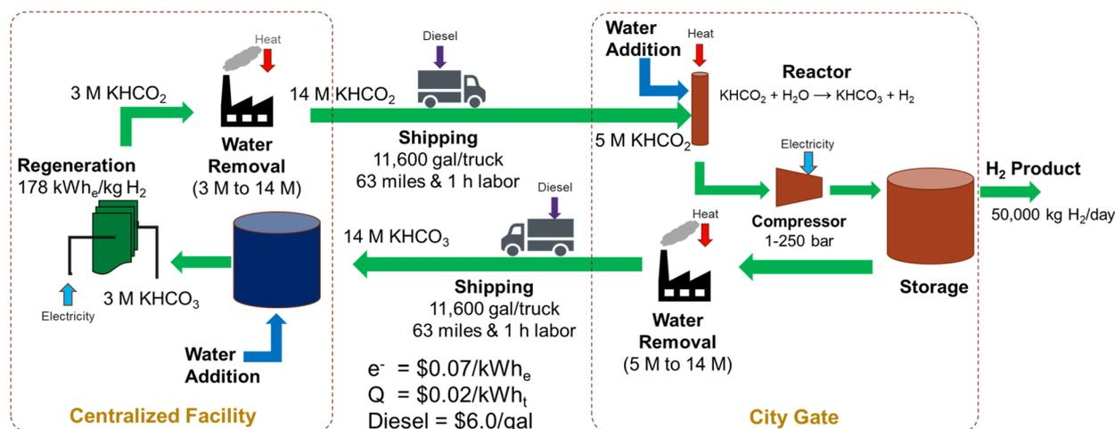
**Fig. 6** Material flow diagram used for an initial cost analysis of the hybrid bicarbonate/formate cycle (electrochemical reduction of bicarbonate coupled with catalytic oxidation of formate to bicarbonate) for a regional refueling depot use case.
