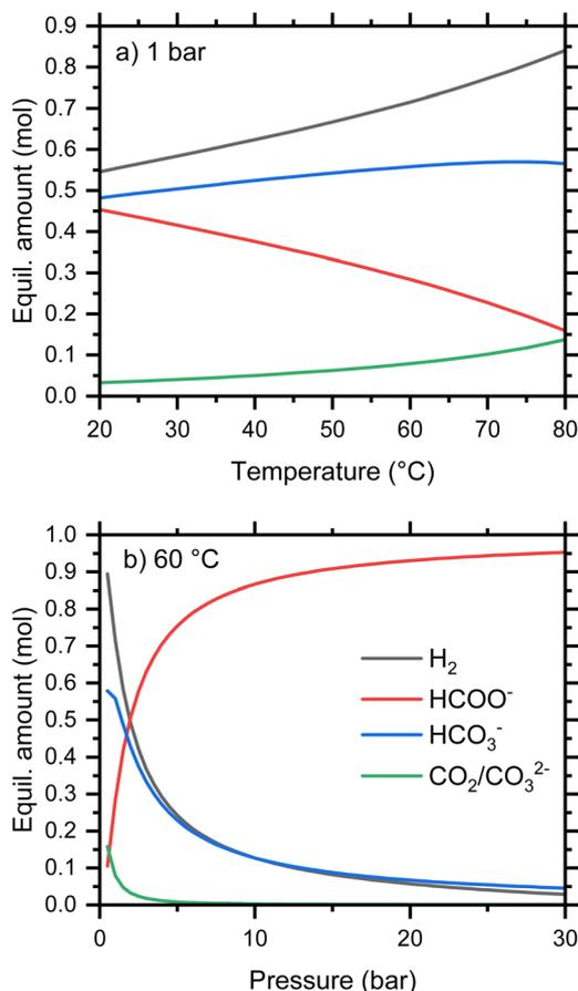
Fig. 3 Calculated equilibrium amounts of selected species from 1 mol KHCO<sub>2</sub> in 1 kg water as a function of (a) pressure, and (b) temperature.
