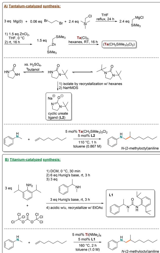
**Scheme 4** Generalized synthetic procedure to produce 1 kg of *N*-(2-methyloctyl)aniline from commercially available starting materials for the tantalum-catalyzed route (A) and the titanium-catalyzed route (B).
