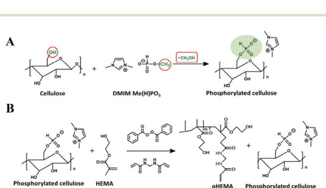
**Fig. 25** (A) Cellulose dissolution and modification in [DMIM][MeO(H)PO<sub>3</sub>] ionic liquid. (B) Polymerisation of HEMA in the presence of phosphorylated cellulose in order to obtain a dual network ionogel. Reproduced from ref. 217 with permission from Elsevier, copyright 2019.
