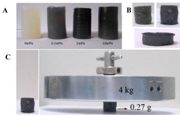
**Fig. 27** (A) Cellulose/reduced graphene oxide (rGO) hydrogels with varying rGO content. (B) Aerogels obtained after freeze-drying process. (C) Demonstration of the mechanical strength of the aerogel. Reproduced from ref. 229 with permission from Elsevier, copyright 2015.
