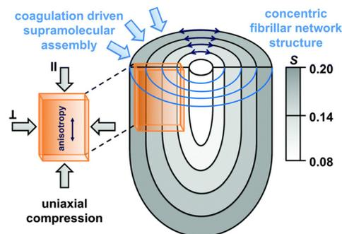
**Fig. 28** Cellulose gel with concentric onion-like layers that have different level of ordering as shown with the *S* parameter, which indicates higher degree of ordering from the core towards the skin layer. Reproduced from ref. 236 with permission from The Royal Society of Chemistry, copyright 2019.
