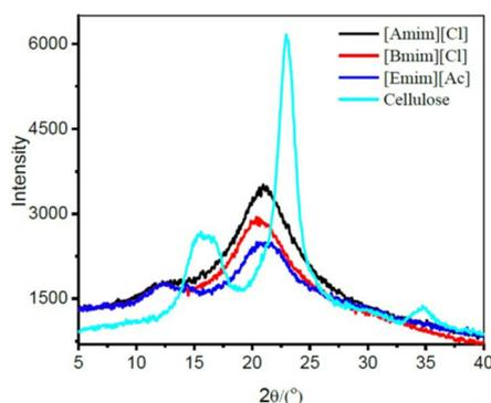
**Fig. 7** X-ray diffraction (XRD) patterns of native cellulose (coniferous dissolving pulp), exhibiting typical cellulose I structure, and that of the films regenerated from different ionic liquids in water with XRD profiles typical for a cellulose II structure. Crystallinity index: [Amim][Cl] > [Bmim][Cl] > [Emim][Ac]. Reproduced from ref. 97 with permission from Elsevier, copyright 2018.
