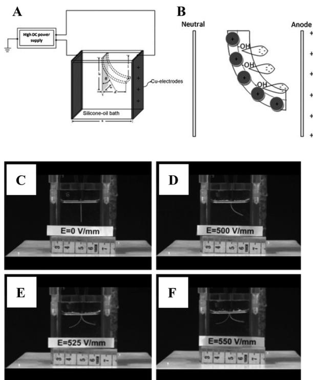
**Fig. 21** (A) Experimental setup for studying the bending response of the ionogel under an applied electric field. (B) Schematic representation of the proposed mechanisms of the bending response. (C and D) Deflection and (E and F) swinging movement of the ionogel in response to a ground and positive electric field at room temperature. Reproduced from ref. 201 with permission from Elsevier, copyright 2012.
