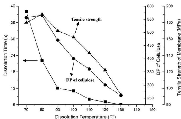
**Fig. 8** Effect of dissolution time and temperature on the tensile strength and degree of polymerisation (DP) of regenerated cellulose (dissolved in [Bmim][Cl], regenerated in water). Reproduced from ref. 95 with permission from Wiley, copyright 2012.
