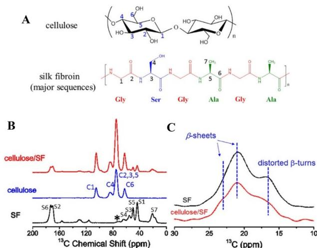
**Fig. 19** (A) Structure of cellulose and silk fibroin with numbering for peak assignment (below). (B)  $^{13}\text{C}$  CP/MAS NMR spectra of regenerated silk fibroin (SF), cellulose and cellulose/silk fibroin composite (3/1). Asterisk indicates spinning sideband. (C)  $^{13}\text{C}$  NMR spectra of regenerated SF and cellulose/SF composite in the Ala  $^{13}\text{C}_\beta$  region for comparison. Reproduced from ref. 180 with permission from the American Chemical Society, copyright 2017.
