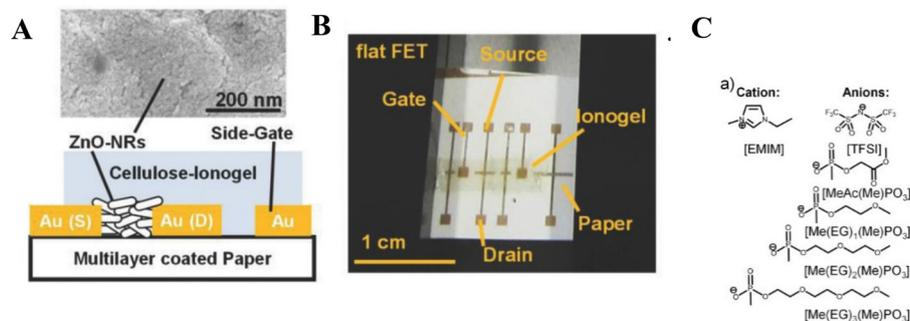
**Fig. 22** (A) The structure of the ionic liquids used to fabricate the ionogels for electrolyte-gated field-effect transistor (FET) devices. (B) Schematic description of the flexible FET device with ZnO nanorods (NRs); an SEM image is shown above the device) and cellulose ionogel. (C) Photograph of the flexible paper-based FET. Reproduced from ref. 202 with permission from Wiley, copyright 2013.
