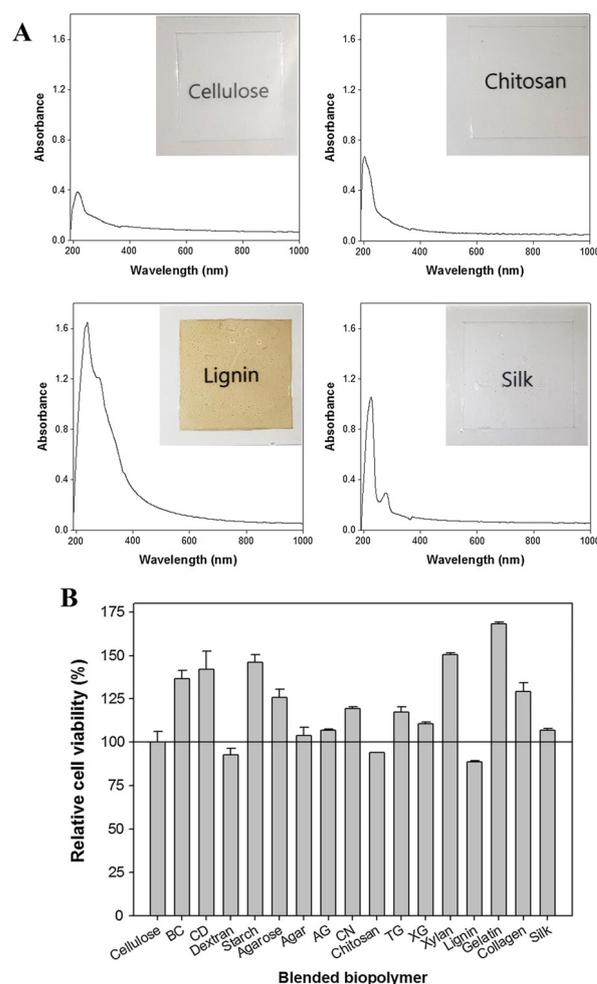
**Fig. 20** (A) UV-Vis spectra of regenerated cellulose, cellulose/chitosan, cellulose/lignin and cellulose/silk films with good light barrier properties below 400 nm. (B) Cell viability of TCMK-1 cells cultured on the composite films. Reproduced from ref. 194 with permission from Springer Nature, copyright 2020.
