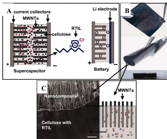
**Fig. 16** (A) Supercapacitor and Li-ion battery device fabricated using the regenerated cellulose/MWCNT composite. (B) Demonstration on the flexibility of the composite film. (C) Cross-sectional SEM image of the nanocomposite film. Reproduced from ref. 150 with permission from the National Academy of Sciences, copyright 2007.
