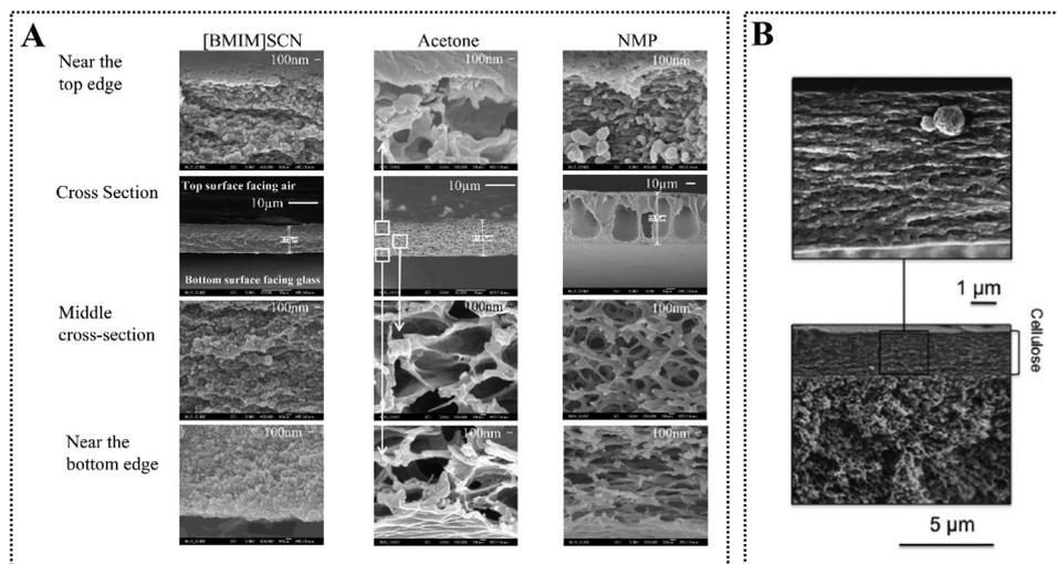
**Fig. 11** (A) Morphology of cellulose acetate membranes regenerated from different solvents (10 wt% cellulose acetate solution). Reproduced from ref. 113 with permission from the American Chemical Society, copyright 2010. (B) Morphology of cellulose membrane on porous polysulphone support regenerated from 10 wt% cellulose solution in [Emim][Ac]. Reproduced from ref. 116 with permission from Elsevier, copyright 2015.
