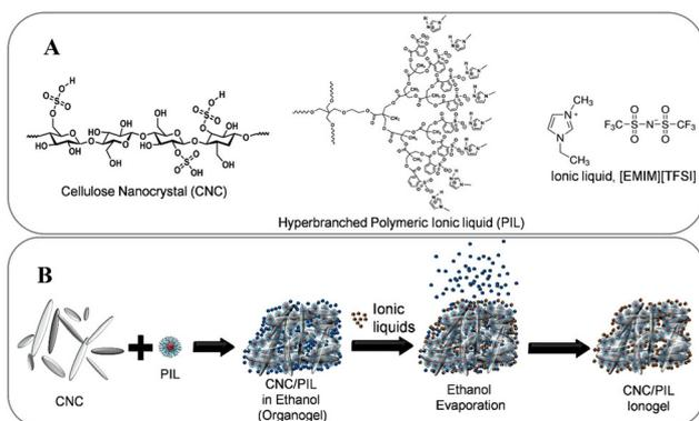
**Fig. 24** (A) Ionogel containing cellulose nanocrystals, hyperbranched polymeric ionic liquid and [Emim][NTf<sub>2</sub>]. (B) Method to prepared the CNC/PIL ionogel containing [Emim][NTf<sub>2</sub>]. Note that TFSI = NTf<sub>2</sub>. Reproduced from ref. 211 with permission from Wiley, copyright 2021.
