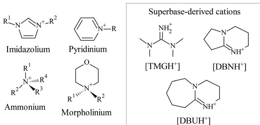
Fig. 4 Typical cations of ionic liquids with ability to dissolve cellulose.
