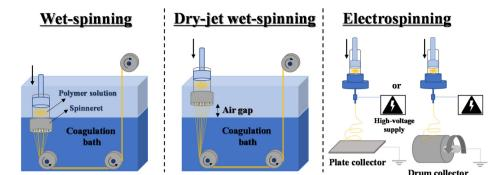
Fig. 29 Common spinning techniques for fabricating synthetic cellulose fibres from solutions. Other methods, such as dry-jet spinning uses no coaqulation bath, and for melt spinning the polymer melt is extruded through the spinneret (note that this is not possible for cellulose itself).
