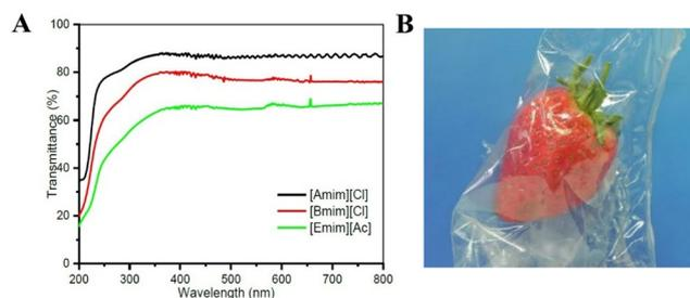
**Fig. 6** (A) Transmittance of cellulose films regenerated from ionic liquids in water as coagulant (the film from [Amim][Cl] has transparency of about 90% at 550 nm). Reproduced from ref. 97 with permission from Elsevier, copyright 2018. (B) Transparent regenerated cellulose film for food packaging application (cotton linter cellulose dissolved in [Emim][Ac], containing 25% glycerol as plasticiser). Reproduced from ref. 98 with permission from Springer Nature, copyright 2013.
