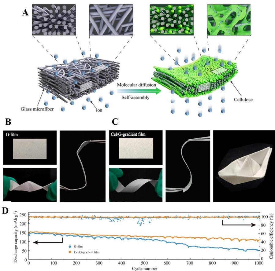
**Fig. 15** (A) Fabrication of cellulose/glass microfiber composite film for application as separator in lithium-batteries. (B) Glass microfiber film with poor flexibility. (C) Cellulose/glass microfiber composite film with excellent flexibility and formability. (D) Cycling stability of a LiFePO<sub>4</sub>/Li cell using glass microfiber (blue line) vs. cellulose/glass microfiber composite (orange line) separators. Reproduced from ref. 149, copyright 2021 The Authors.
