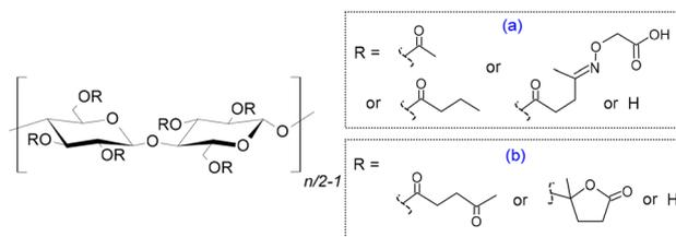
**Fig. 5** Mixed cellulose ester obtained by using levulinic acid and acyl anhydrides as reactants, followed by the reaction of the corresponding mixed ester with (aminoxy)acetic acid to afford the water-dispersible derivative (a);<sup>76</sup> and obtained through alpha-angelica lactone in 1,8-diazabicyclo[5.4.0]undec-7-ene ([DBU])/dimethyl sulfoxide/carbon dioxide organocatalytic system (b).<sup>77</sup>
