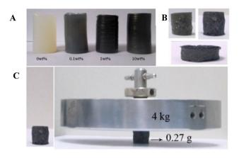
Fig. 27 (A) Cellulose/reduced graphene oxide (rGO) hydrogels with varying rGO content. (B) Aerogels obtained after freeze-drying process. (C) Demonstration of the mechanical strength of the aerogel. Reproduced from ref. 229 with permission from Elsevier, copyright 2015.
