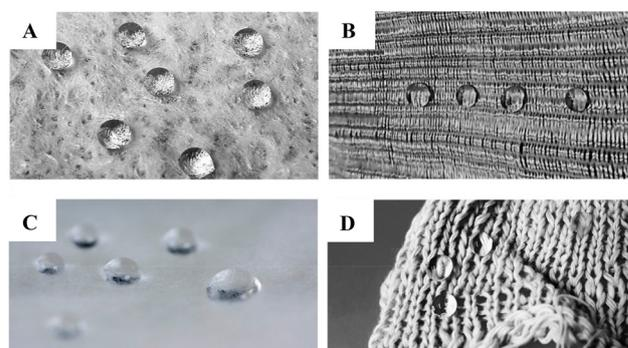
**Fig. 31** Hydrophobic Ioncell-F fibres with 10 wt% (A and B) betulin and betulinic acid (C and D). Left pictures are nonwovens, right pictures are hand loomed/knitted fabrics. Reproduced from ref. 294, copyright 2021 The Authors.
