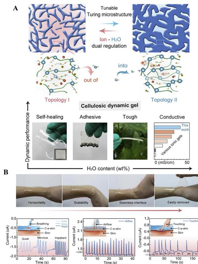
**Fig. 23** (A) Transition between two topological networks by adjusting the water content of a cellulose/[Bmim][Cl] ionogel. The ionogel thus exhibits tunable dynamic properties as shown in the bottom of the figure. (B) Application of the dynamic ionogel in an electronic skin device that can be used for sensing *e.g.*, breathing pattern, airflow and touching. Reproduced from ref. 205 with permission from Elsevier, copyright 2019.
