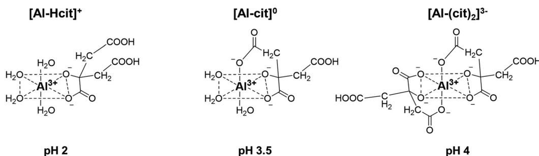
Fig. 2 Structures of different Al-citrate complexes and pH values at which their presence is most dominant.<sup>50,51</sup>
