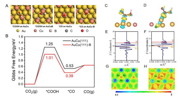
Fig. 5 (A) Adsorption configurations of \*COOH and \*CO on AuCu(111) and AuCu(111)-B. (B) Gibbs free energy profiles for CO₂RR on AuCu(111) and AuCu(111)-B. Charge density difference plots of \*COOH adsorption on AuCu(111) (C) and AuCu(111)-B (D). Planar-averaged charge density difference of \*COOH adsorption on AuCu(111) (E) and AuCu(111)-B (F). Surface electrostatic potentials of AuCu(111) (G) and AuCu(111)-B (H).
