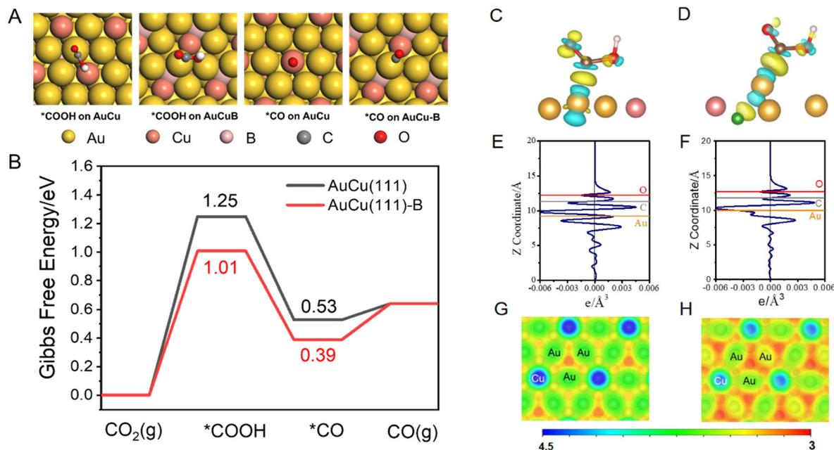
Fig. 5 (A) Adsorption configurations of \*COOH and \*CO on AuCu(111) and AuCu(111)-B. (B) Gibbs free energy profiles for CO<sub>2</sub>RR on AuCu(111) and AuCu(111)-B. Charge density difference plots of \*COOH adsorption on AuCu(111) (C) and AuCu(111)-B (D). Planar-averaged charge density difference of \*COOH adsorption on AuCu(111) (E) and AuCu(111)-B (F). Surface electrostatic potentials of AuCu(111) (G) and AuCu(111)-B (H).
