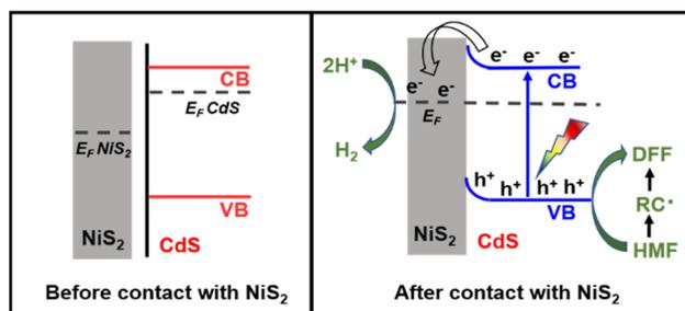
**Scheme 2** Energy band diagrams of the pure CdS and NiS<sub>2</sub>/CdS before contact with metallic NiS<sub>2</sub> and the interfacial photoinduced charge transfer and reaction after contact with NiS<sub>2</sub> and light irradiation.
