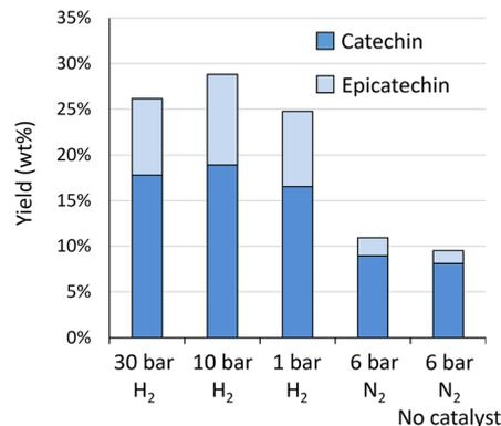
**Fig. 6** Influence of H<sub>2</sub> pressure (at RT) on the depolymerisation–hydrogenation of procyanidins. Reaction conditions: 200 mg Oligopin, 60 mL methanol, 1–30 bar H<sub>2</sub> or 6 bar N<sub>2</sub>, 25 mg Pd/C (or no catalyst), 3 h reaction time.
