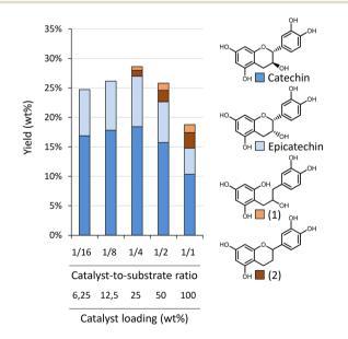
Fig. 5 Influence of catalyst loading (with respect to substrate) on the depolymerisation-hydrogenation of procyanidins. Reaction conditions: 200 mg Oligopin, 60 mL methanol, 30 bar H<sub>2</sub>, varying catalyst loading (from 12.5 to 200 mg Pd/C), 3 h reaction time. Next to (epi)catechin, also hydrogenation products were detected: a ring opened catechin (1) and a dehydroxylated catechin (2).
