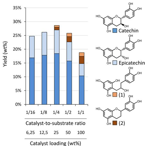
**Fig. 5** Influence of catalyst loading (with respect to substrate) on the depolymerisation–hydrogenation of procyanidins. Reaction conditions: 200 mg Oligopin, 60 mL methanol, 30 bar H<sub>2</sub>, varying catalyst loading (from 12.5 to 200 mg Pd/C), 3 h reaction time. Next to (*epi*)catechin, also hydrogenation products were detected: a ring opened catechin (1) and a dehydroxylated catechin (2).
