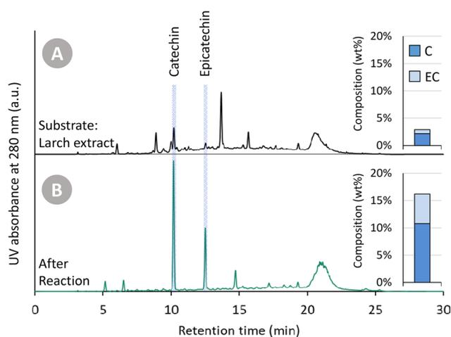
**Fig. 7** HPLC-UV analysis and quantification of catechin (C) and epicatechin (EC) of two solutions: (A) crude larch bark extract, as obtained via Soxhlet extraction with methanol, and (B) the product mixture after depolymerisation–hydrogenation of a crude larch bark extract. Reaction conditions: 60 mL crude larch bark extract in methanol (4.8 g extractives per L), 30 bar H<sub>2</sub>, 25 mg Pd/C, 200 min reaction time.
