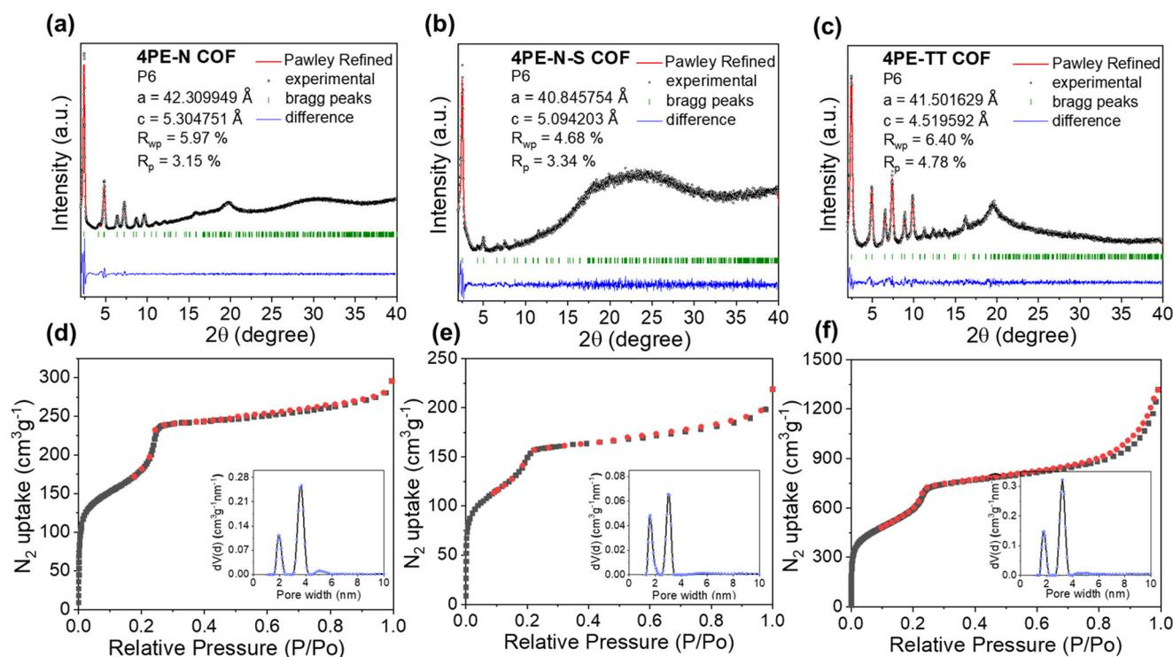
Fig. 2 The PXRD patterns and Pawley refinements of (a) 4PE-N-COF, (b) 4PE-N-S-COF and (c) 4PE-TT-COF. N<sub>2</sub> adsorption/desorption isotherms and pore size distributions (inset) of (d) 4PE-N-COF, (e) 4PE-N-S-COF and (f) 4PE-TT-COF.
