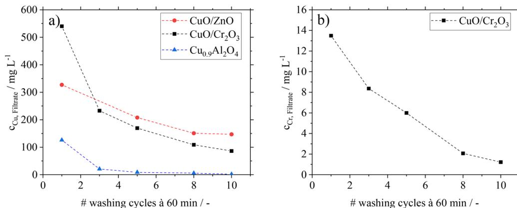
**Fig. 3** Metal leaching from different Cu-based catalysts over ten washing cycles using FA–MF mixtures as washing solution (scenario B); filtrate solutions analyzed by ICP-OES: (a) Cu leaching; (b) Cr leaching for CuO/Cr<sub>2</sub>O<sub>3</sub>.
