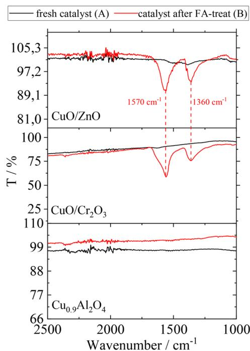
**Fig. 4** ATR-IR spectra of CuO/ZnO, CuO/Cr<sub>2</sub>O<sub>3</sub> and  $\text{Cu}_{0.9}\text{Al}_2\text{O}_4$  before (A) and after (B) contact with FA; assignment of peaks: carboxylate ion of formate species (1570  $\text{cm}^{-1}$  asymmetric stretch and 1360  $\text{cm}^{-1}$  symmetric stretch).<sup>33</sup>
