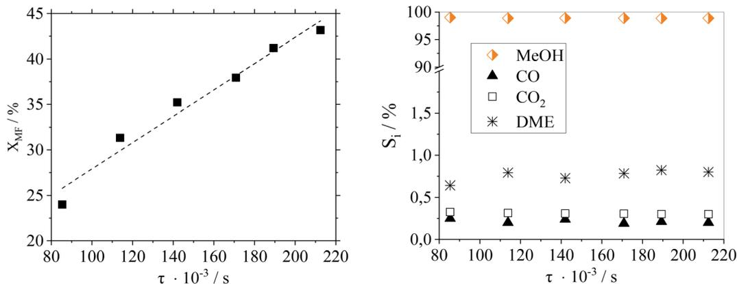
Fig. 7 Effect of residence time variation on (a) conversion and (b) selectivity in pure MF hydrogenolysis using Cu<sub>0.9</sub>Al<sub>2</sub>O<sub>4</sub>; reaction conditions:  $p = 10$  bar<sub>g</sub>,  $T = 188$  °C,  $n_{\text{H}_2} : n_{\text{MF}}^{-1} = 5.6$ ,  $V_{\text{total}} = 566\text{--}1408$  ml<sub>N</sub> min<sup>-1</sup>,  $m_{\text{cat.}} = 0.32$  g.
