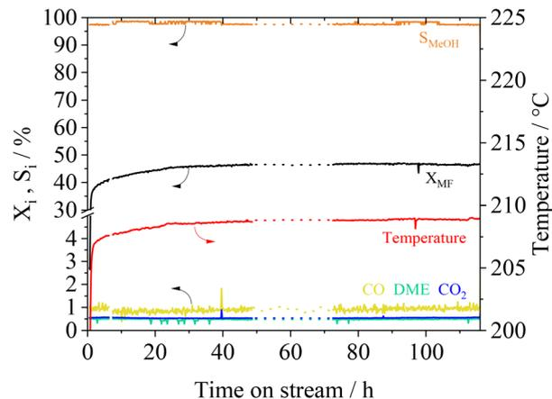
Fig. 8 Conversion and selectivity over time with the Cu<sub>0.9</sub>Al<sub>2</sub>O<sub>4</sub> catalyst, reaction conditions:  $T = 208$  °C,  $p = 10$  bar<sub>g</sub>,  $V_{\text{total}} = 704$  ml<sub>N</sub> min<sup>-1</sup>,  $n_{\text{H}_2} : n_{\text{MF}} = 5.8$ ,  $m_{\text{cat.}} = 0.5$  g; dotted line: interpolation of experimental data during a temporal breakdown of our reaction analytics.
