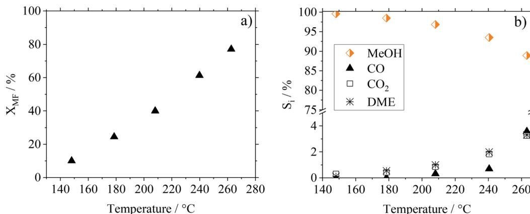
**Fig. 6** Temperature influence on (a) conversion and (b) selectivity in pure MF hydrogenolysis using Cu<sub>0.9</sub>Al<sub>2</sub>O<sub>4</sub>; reaction conditions:  $T = 150\text{--}260 \text{ °C}$ ,  $p = 10 \text{ bar}_g$ ,  $V_{\text{total}} = 704 \text{ mL}_N \text{ min}^{-1}$ ,  $n_{H_2} : n_{MF} = 5.8$ ,  $m_{\text{cat.}} = 0.5 \text{ g}$ .
