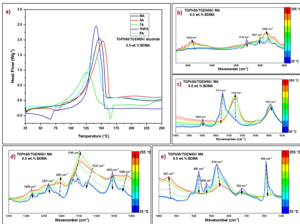
**Fig. 2** (a) Dynamic DSC thermograms obtained during the crosslinking of TGPh50/TGEN50//anhydride formulations initiated by 0.5 wt% BDMA, and the temperature-dependent FT-IR spectra of the TGPh50/TGEN50//MA system during curing in the regions (b) 3800–2800  $\text{cm}^{-1}$ , (c) 1950–1550  $\text{cm}^{-1}$ , (d) 1350–1000  $\text{cm}^{-1}$ , and (e) 1000–650  $\text{cm}^{-1}$ .
