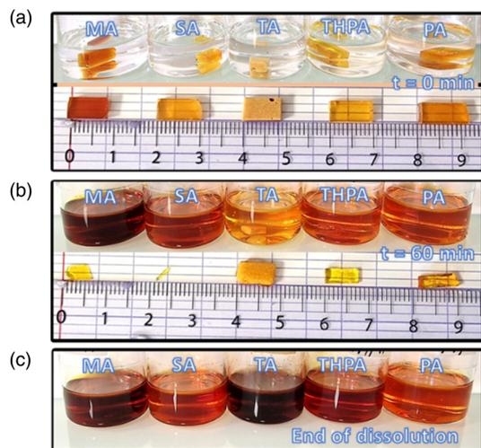
**Fig. 5** Physical appearance of the thermosets during immersion in TBD-EG solution at 170 °C: (a)  $t = 0$  min; (b)  $t = 60$  min; (c) end of dissolution at  $t = 70$  min for MA & SA systems, at  $t = 150$  min for THPA & PA systems and  $t = 12$  h 30 min for the TA system.
