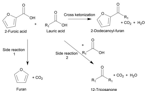
**Fig. 2** Scheme for the overall ketonization reaction between 2-furoic acid and lauric acid ( $R_1 = C_{11}H_{23}$ ). The side reactions 1 and 2 are the decarboxylation of 2-furoic acid to furan and the lauric acid self-ketonization to 12-tricosanone.
