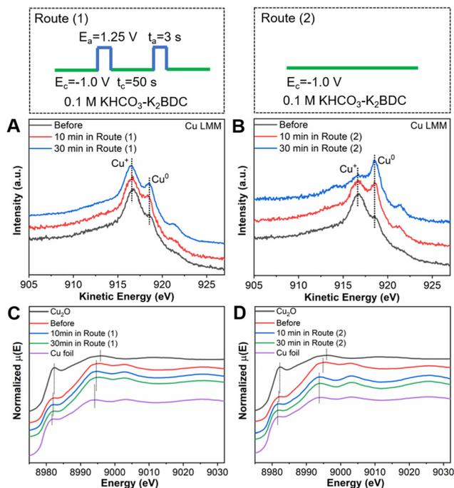
**Fig. 3** The quasi *in situ* Auger LMM spectra of Cu for Cu<sub>x</sub>C<sub>y</sub>O<sub>z</sub>(0.41) reacted in (A) route (1) and (B) route (2) for different times. The *in situ* XANES spectra of Cu<sub>x</sub>C<sub>y</sub>O<sub>z</sub>(0.41) reacted in (C) route (1) and (D) route (2) for different times.
