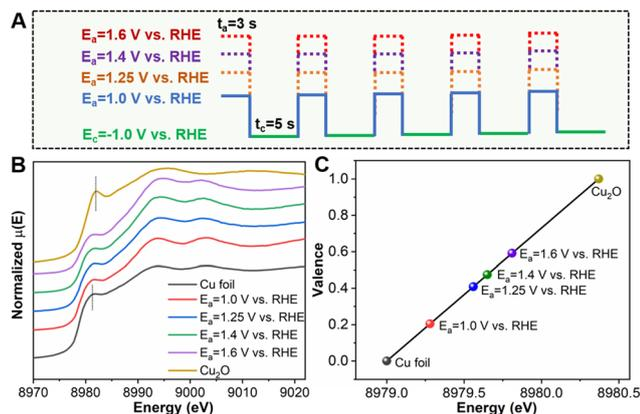
**Fig. 2** (A) Schematic diagram of the preparation of the Cu<sub>x</sub>C<sub>y</sub>O<sub>z</sub> catalyst under different conditions ( $E_a = 1.0$  V, 1.25 V, 1.4 V, and 1.6 V vs. RHE,  $t_a = 3$  s,  $E_c = -1.0$  V vs. RHE,  $t_c = 5$  s). (B) XANES spectra at the Cu K-edge under different conditions. (C) Average oxidation state of Cu in Cu<sub>x</sub>C<sub>y</sub>O<sub>z</sub> under different conditions from Cu K-edge XANES.
