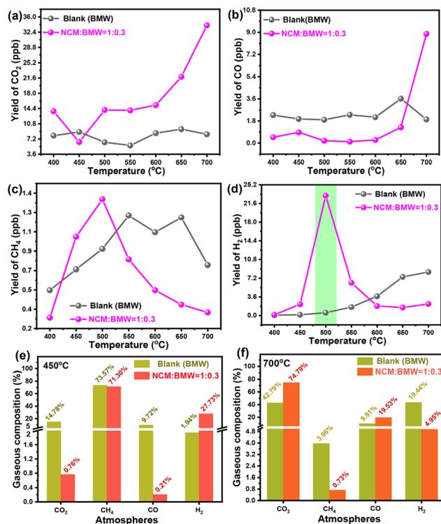
Fig. 4 Analytical results of GC: the yield of different gases from the blank sample and the mixed sample at different temperatures (a)  $\text{CO}_2$ ; (b)  $\text{CO}$ ; (c)  $\text{CH}_4$ ; (d)  $\text{H}_2$ ; (e)  $450\text{ }^{\circ}\text{C}$ ; (f)  $700\text{ }^{\circ}\text{C}$ .
