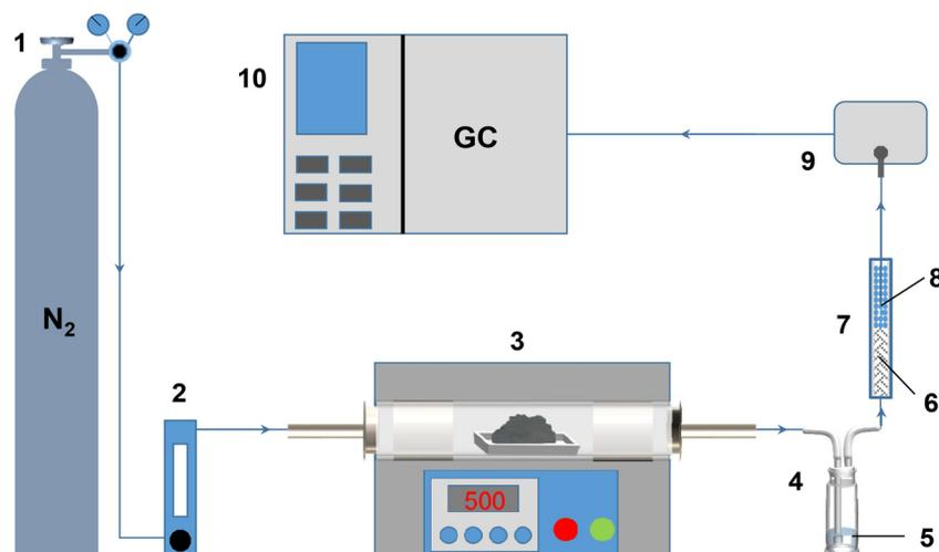
**Fig. 1** The self-designed equipment for the thermochemical experiment (1. Nitrogen cylinder, 2. Gas flowmeter, 3. Glass tube furnace, 4. Gas-washing system, 5. Saturated sodium bicarbonate, 6. Skimmed cotton, 7. Drying tube, 8. Discolored silica gel, 9. Gas sample collection bag, 10. Gas chromatograph instrument).
