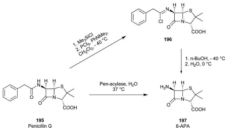
Fig. 50 Conventional chemical vs. enzymatic deacylation of penicillin G.<sup>209</sup>
