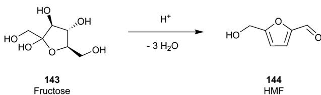
Fig. 34 Acid-catalysed formation of HMF by dehydrogenation of fructose.<sup>165</sup>
