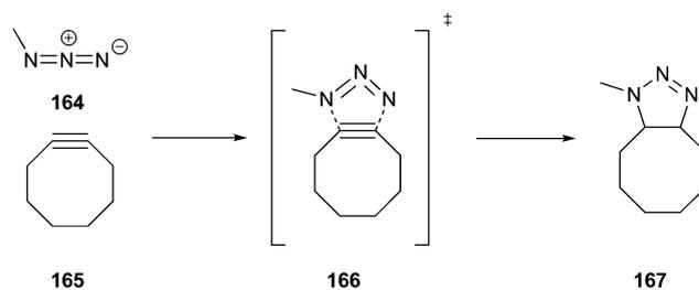
Fig. 41 General mechanism of SPAAC.<sup>181</sup>
