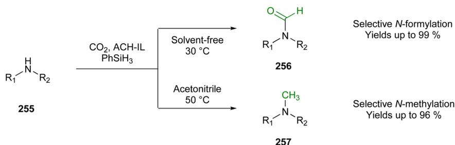
Fig. 66 Safe solvent- and temperature-controlled *N*-functionalization with CO<sub>2</sub> and ACH-ILs by Zhao *et al.*<sup>330</sup>
