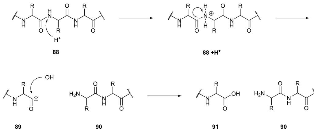
Fig. 22 Cleavage mechanism of peptide bonds in subcritical water.<sup>142</sup>
