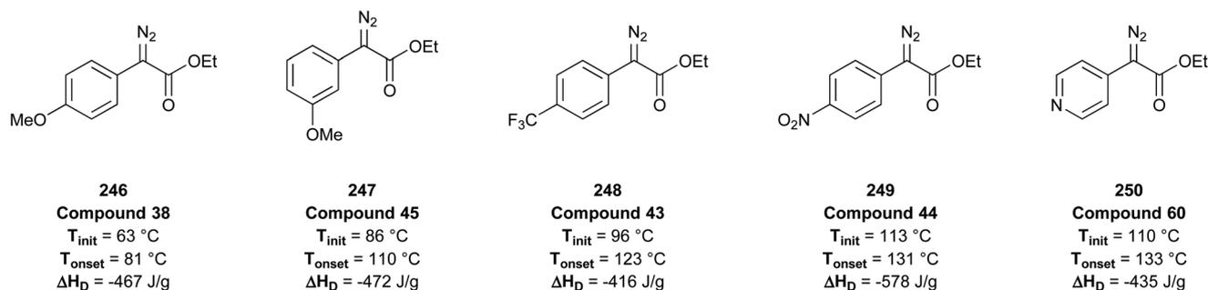
Fig. 63 Thermal assessment of selected diazo compounds by Green *et al.*<sup>321</sup>
