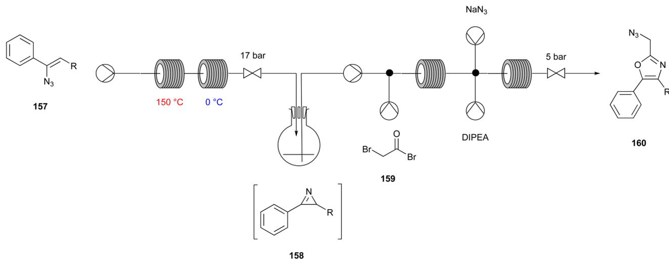
Fig. 39 Continuous-flow synthesis of 2-(azidomethyl)oxazoles.<sup>176</sup>
