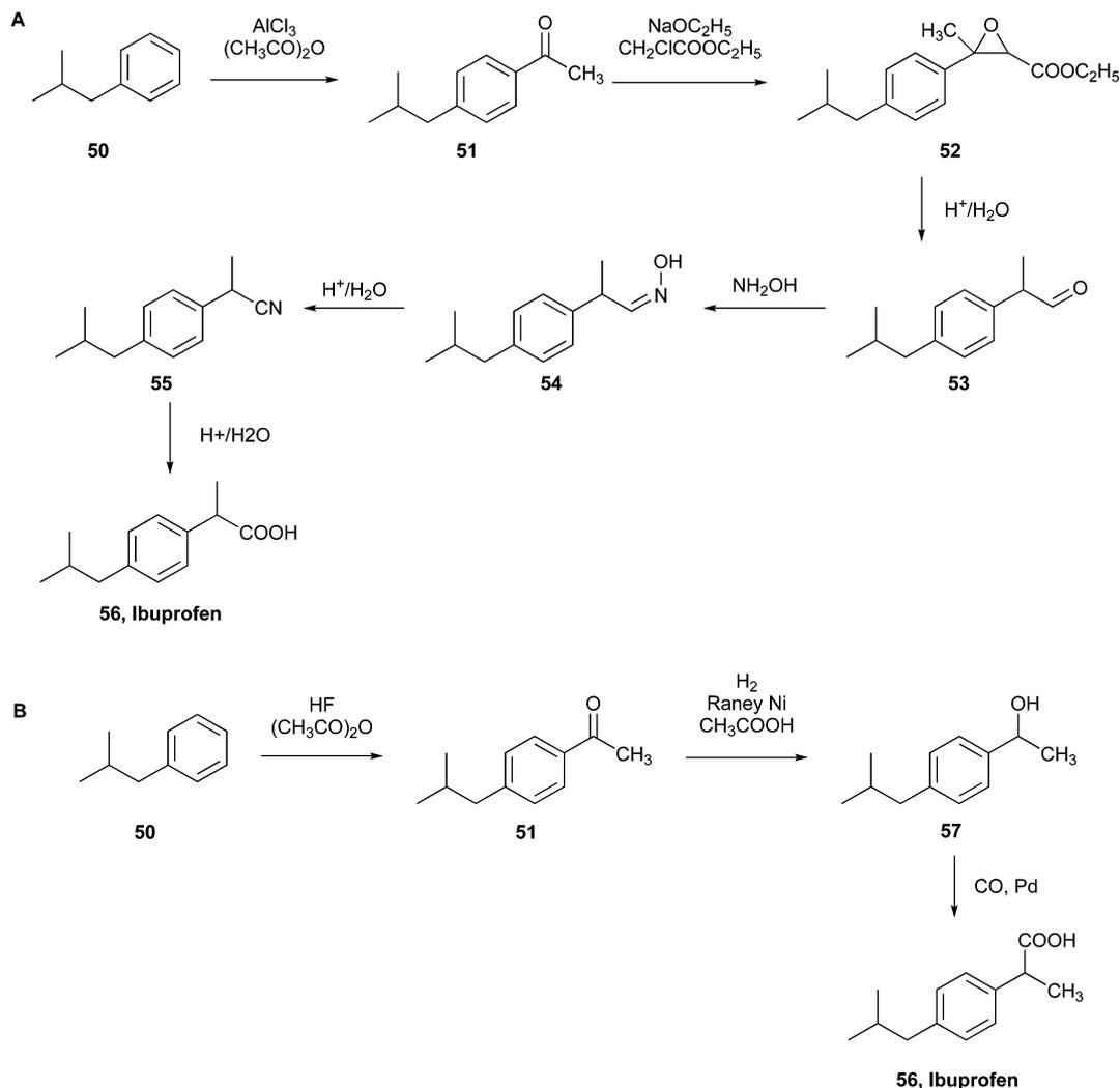
Fig. 15 (A) Boots initial commercial synthesis of ibuprofen.<sup>103</sup> (B) BHC Company new commercial green synthesis of ibuprofen.<sup>104</sup>
