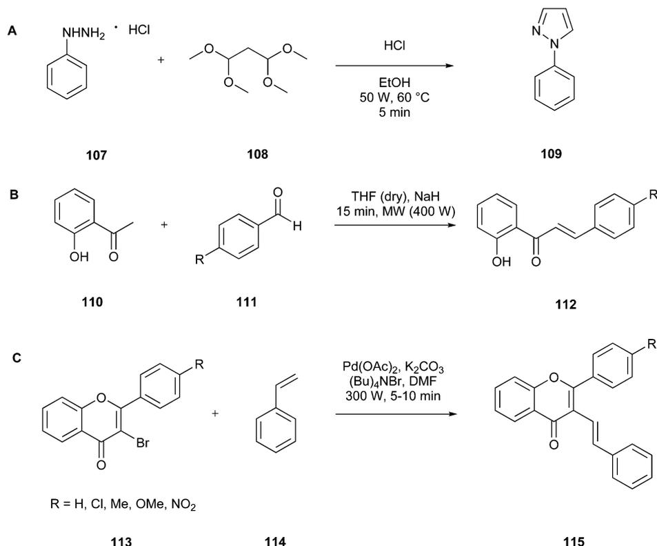
**Fig. 27** (A) Microwave-assisted synthesis of phenyl-1H-pyrazole.<sup>18</sup> (B) Aldol-condensation of the example of 2'-hydroxyacetophenone under MW.<sup>151</sup> (C) Synthesis of (*E*)-3-styrylflavones.<sup>152</sup>
