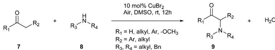
Fig. 3 One-step synthesis between  $\alpha$ -carbonyls and functionalised amines.<sup>4</sup>
