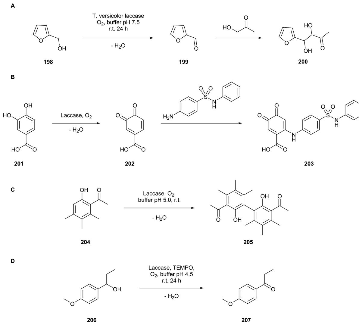
Fig. 51 Examples of laccase-catalysed (A) aldol addition, (B) Michael reaction, (C) dimerisation, and (D) chemoenzymatic oxidation with TEMPO.<sup>211,214</sup>
