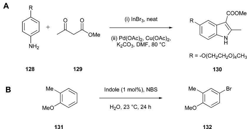
Fig. 31 (A) Synthesis of indole compound used as PTCat.<sup>159</sup> (B) Bromination with PTCat.<sup>159</sup>
