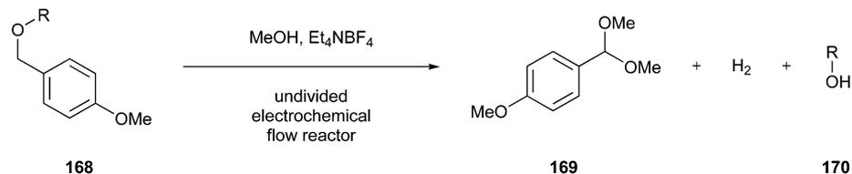
Fig. 42 Electrochemical deprotection of *para*-methoxybenzyl ethers.<sup>187</sup>
