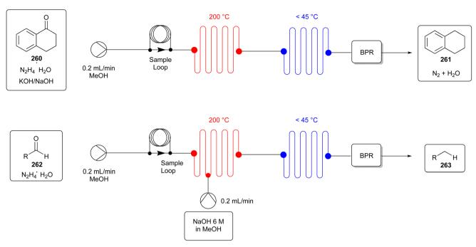
Fig. 68 Safer Wolff–Kishner reduction of ketones/aldehydes in flow-chemistry conditions. 333,335
