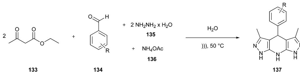
Fig. 32 One-pot synthesis of pyrazole-derivatives.<sup>161</sup>
