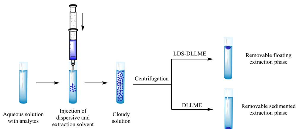
Fig. 62 Schematic general process of DLLME and LDS-DLLME.<sup>278</sup>
