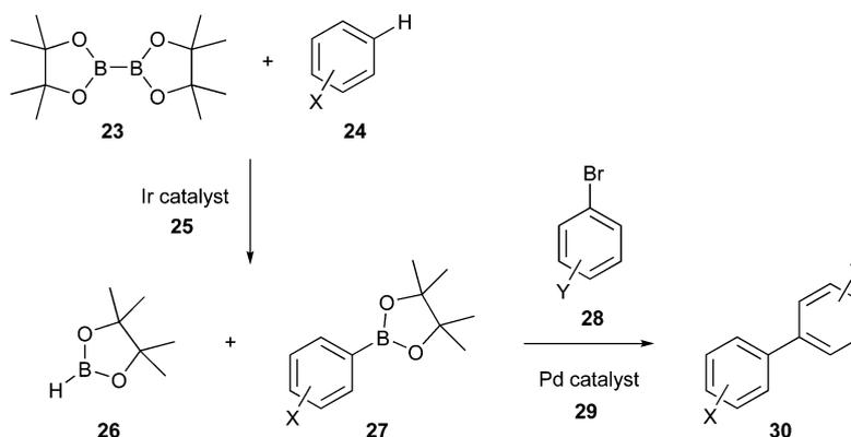
Fig. 10 'One-pot' *in situ* borylation by C–H activation for greener Suzuki process.<sup>85</sup>
