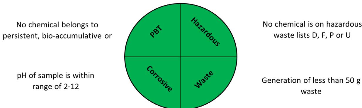
Fig. 60 General description of National Environmental Method Index.<sup>268</sup>
