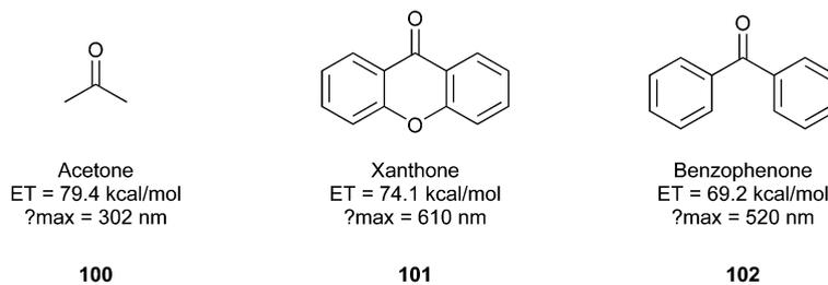
Fig. 25 Photosensitiser with triplet state energies ( $E_T$ ) and absorbance ( $\lambda_{max}$ ).<sup>148</sup>
