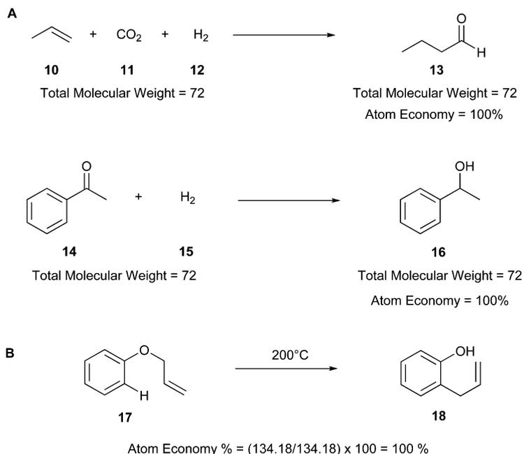
Fig. 4 (A) Examples of theoretical calculation of atom economy.<sup>20</sup> (B) Atom economy of the Claisen rearrangement reaction.<sup>40</sup>
