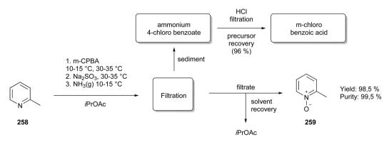
Fig. 67 m-CPBA-system for the secure manufacturing of N-oxides (259).<sup>332</sup>
