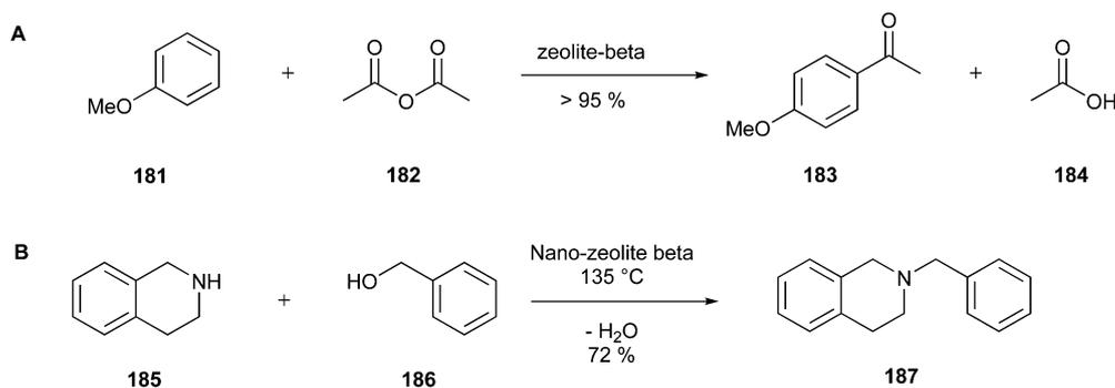
Fig. 47 (A) Zeolite-catalysed acylation of anisole by Rhône Poulenc.<sup>188</sup> (B) *N*-Alkylation with nanosized zeolite-catalysis.<sup>204</sup>
