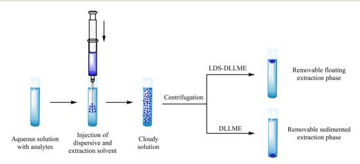
Fig. 62 Schematic general process of DLLME and LDS-DLLME.<sup>278</sup>
