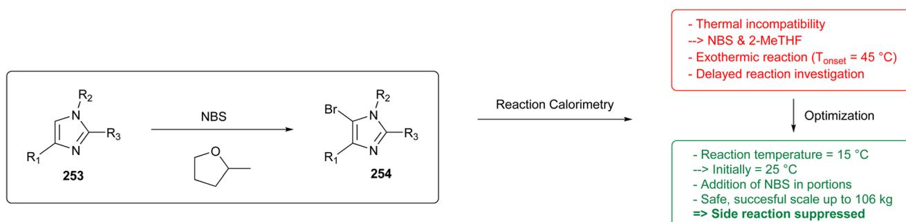
Fig. 65 Optimization of NBS/2-MeTHF-incompatibility in bromination process.<sup>325</sup>
