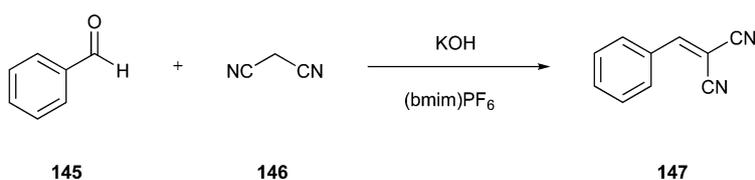
Fig. 35 Knoevenagel condensation of benzaldehyde with malononitrile.<sup>172</sup>
