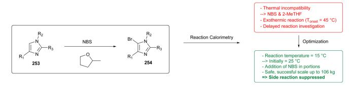
Fig. 65 Optimization of NBS/2-MeTHF-incompatibility in bromination process. 325
