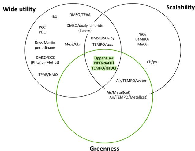
Fig. 7 Venn diagram of oxidation of secondary alcohols to ketones following Pfizer reagent guide.<sup>10</sup>
