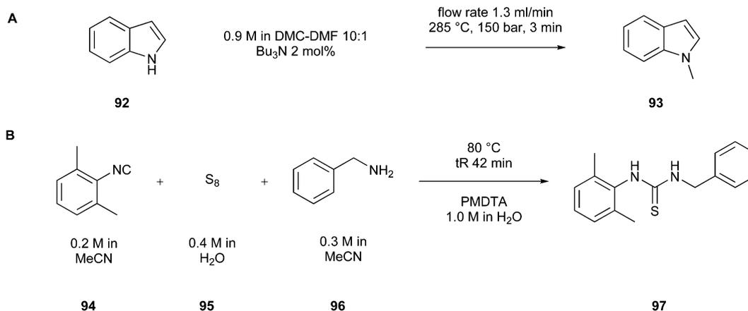
**Fig. 23** (A) Flow-chemistry-based implementation of indole synthesis.<sup>146</sup> (B) Continuous-flow synthesis of 1-benzyl-3-(2,6-dimethylphenyl)thiourea (97).<sup>147</sup>
