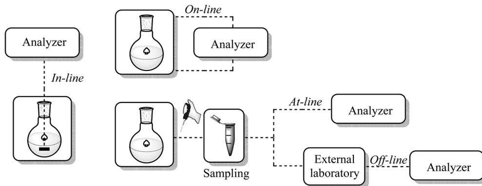
Fig. 59 Measurement variations for analytical investigation.<sup>265</sup>
