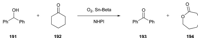
Fig. 49 One-pot BVO of cyclohexanone *via* Sn-beta-zeolite and *in situ*-generated H<sub>2</sub>O<sub>2</sub>.<sup>207</sup>
