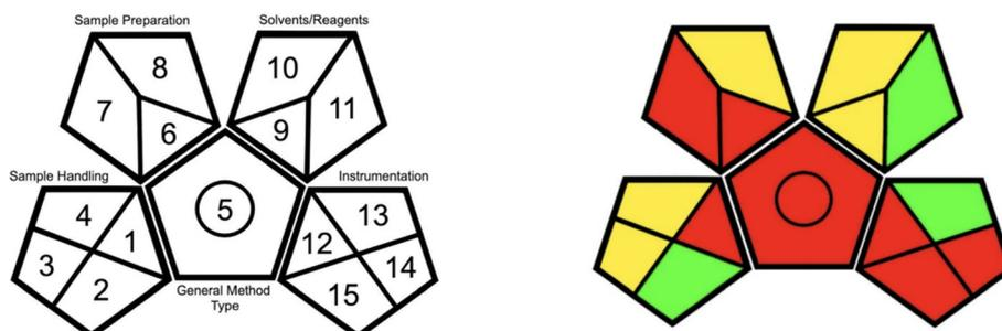
Fig. 61 Composition of GAPI pictogram (left) and evaluation of LLE (right).<sup>25</sup>
