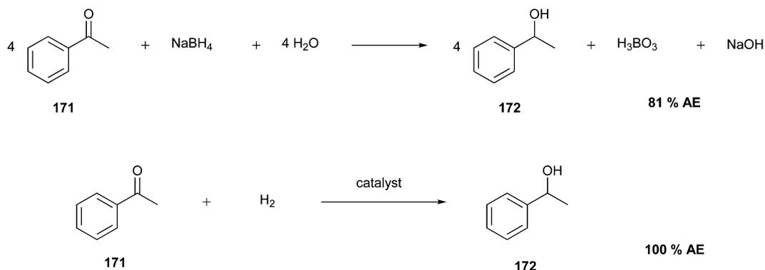
Fig. 43 Reduction with metal hydrides and catalytic hydrogenation.<sup>189</sup>
