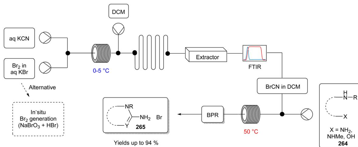
Fig. 69 Continuous-flow synthesis of cyclic guanidines (**265**) with the *in situ* generation of cyanogen bromide.<sup>336</sup>
