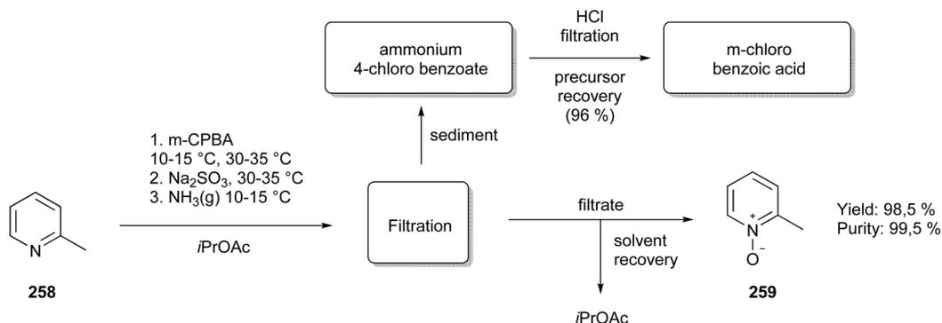
Fig. 67 *m*-CPBA-system for the secure manufacturing of *N*-oxides (**259**).<sup>332</sup>
