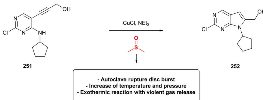
Fig. 64 Rupture disc burst reported by Tian *et al.* due to thermal decomposition of DMSO.<sup>324</sup>
