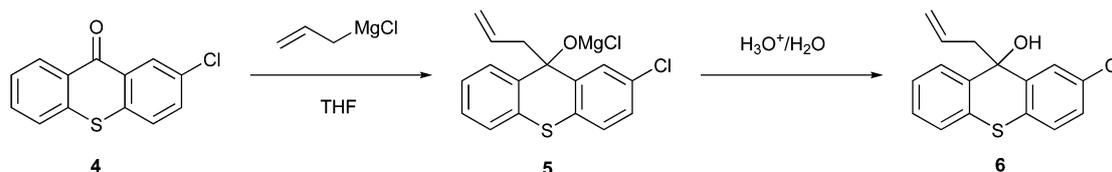
Fig. 2 Synthesis of 9-allyl-2-chloro-9H-thioxanthen-9-ol via continuous processing.<sup>4</sup>
