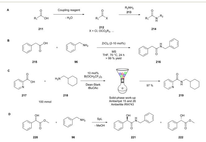
Fig. 53 (A) Direct amidation *via* acid-activation and following amine-coupling.<sup>222</sup> (B) Amide bond formation *via* Zr-catalysis by Adolfsson *et al.*<sup>223</sup> (C) Large-scale boron-catalysed amide-synthesis in *tert*-butyl acetate by Sheppard *et al.* involving Dean–Stark water removal and solid-phase work-up.<sup>224</sup> (D) Enantioselective synthesis of chiral (*R*)-amides *via* SpL.<sup>225</sup>
