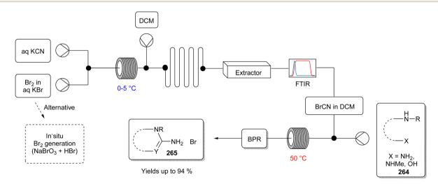
Continuous-flow synthesis of cyclic guanidines (265) with the *in situ* generation of cyanogen bromide. 336
