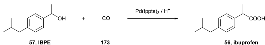
Fig. 44 Carbonylation of IBPE to ibuprofen via water-soluble Pd(tppts) catalyst. 195
