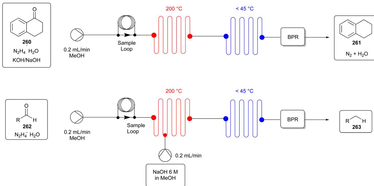
Fig. 68 Safer Wolff–Kishner reduction of ketones/aldehydes in flow-chemistry conditions.<sup>333,335</sup>
