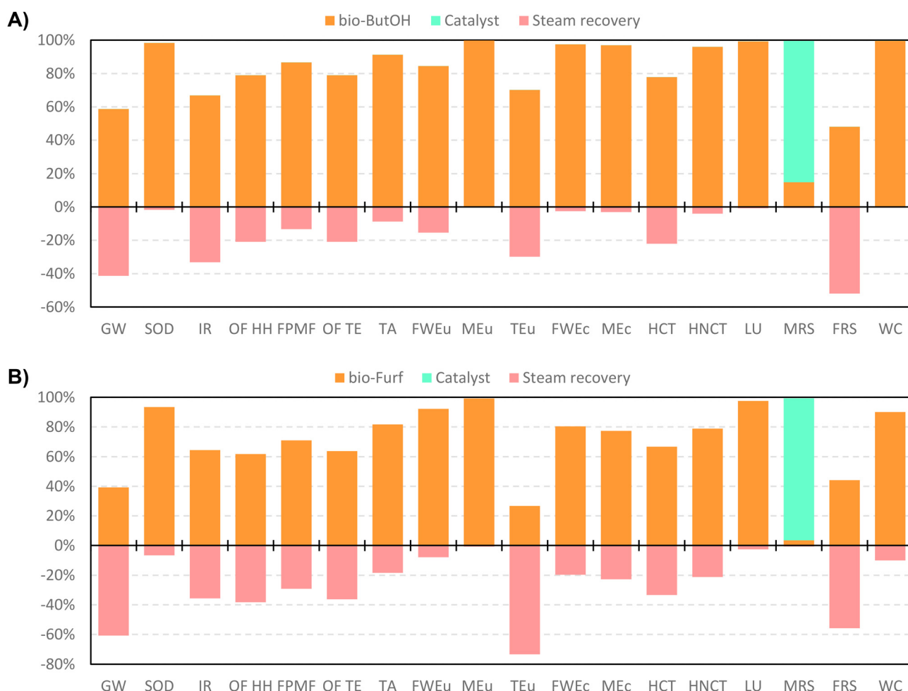
Fig. 7 Contribution analysis of bio-ButOH MA + En.Recov. (A) and bio-Furf MA + En.Recov. (B) using the ReCiPe 2016 method (v.1.07).
