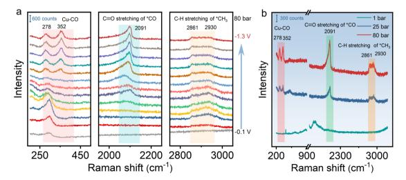
Fig. 3 In situ Raman spectra of HS-Cu obtained (a) in the potential range of -0.1 to -1.3 V vs. Ag/AgCl during the CO<sub>2</sub>RR at 80 bar CO<sub>2</sub> pressure, (b) at different CO<sub>2</sub> pressures during the CO<sub>2</sub>RR at a controlled potential of -1.0 V vs. Ag/AgCl.
