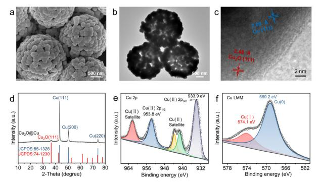
Fig. 1 Characterization of the as-prepared HS-Cu catalyst. (a) SEM image, (b and c) HRTEM image, (d) XRD pattern, (e and f) XPS Cu 2p and Cu LMM Auger electron spectra of Cu₂O@Cu.
