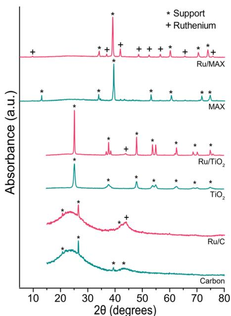
**Fig. 13** X-ray diffraction (XRD) spectra of Ti<sub>3</sub>(Al<sub>0.8</sub>Sn<sub>0.2</sub>)C<sub>2</sub> MAX-phase and Ru/Ti<sub>3</sub>(Al<sub>0.8</sub>Sn<sub>0.2</sub>)C<sub>2</sub> MAX (5 wt%), TiO<sub>2</sub> and Ru/TiO<sub>2</sub> (5 wt%), Carbon and Ru/Carbon (5 wt%). The diffractograms were measured from 5 or 15 to 80 degrees with a scan rate of 1°/minute. The diffraction peaks were assigned using a spectral database within the Rigaku PDXL software.
