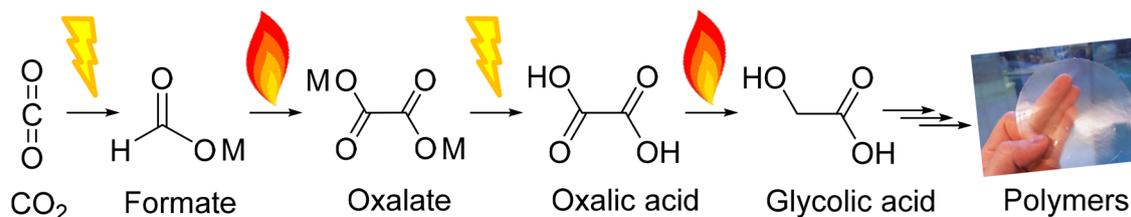
**Fig. 1** "OCEAN" process for CO<sub>2</sub> utilization via (i) electrochemical reduction to formate, (ii) thermal formate coupling to oxalate, (iii) electrochemical oxalate acidification, (iv) thermocatalytic reduction of oxalic acid to glycolic acid, and (v) polymer production from oxalic acid and its derivatives.
