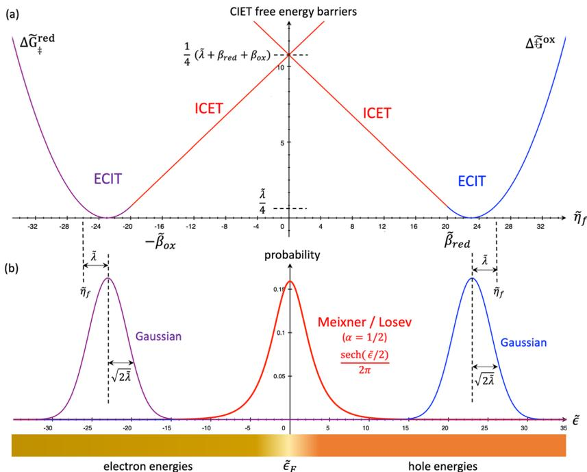
Fig. 12 Quantum statistics of transferring electron energies for symmetric ICET at a metal electrode. (a) Uniformly valid approximation of the CIET energy barriers for  $\tilde{\beta}_{red} = \tilde{\beta}_{ox} = 20$  and  $\tilde{\lambda} = 3$ , and (b) corresponding electron energy distributions for  $\tilde{\eta}_f = -26, 0, 26$ .
