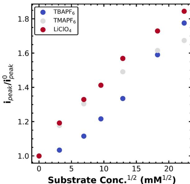
Fig. 4 Normalized peak currents at  $-1.55$  V vs.  $Fc^{+/0}$  for 1 mM FeCl(TPP) in a DMF solution containing 0.1 M TBAPF<sub>6</sub> (blue), TMAPF<sub>6</sub> (grey), or LiClO<sub>4</sub> (red) for increasing amounts of the substrate PhEtCl. Scan rate was 10 mV s<sup>-1</sup> with a 0.07 cm<sup>2</sup> glassy carbon working electrode.
