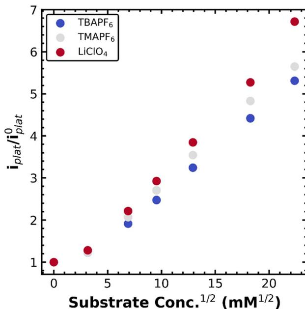
Fig. 2 Normalized plateau currents at  $-1.7 \text{ V vs. Fc}^{+/0}$  for  $1 \text{ mM Co(TPP)}$  in a DMF solution containing  $0.1 \text{ M TBAPF}_6$  (blue),  $0.1 \text{ M TMAPF}_6$  (grey), or  $0.1 \text{ M LiClO}_4$  (red) for increasing amounts of the substrate PhEtCl. Scan rate was  $10 \text{ mV s}^{-1}$  with a  $0.07 \text{ cm}^2$  glassy carbon working electrode.
