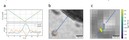
Fig. 5 Pinning of the nanodroplet. (a) Evolution of the applied potential (top, green) and of the displacement (with respect to its initial position) along the normal and tangential direction of the Pt NP discussed in Fig. 1 (bottom) over time. The directions are defined in (b) compared to the reservoir's contact line passing through the NP's initial centre of mass. (c) Trajectory of the Pt NP with a colour scale conveying its optical intensity.
