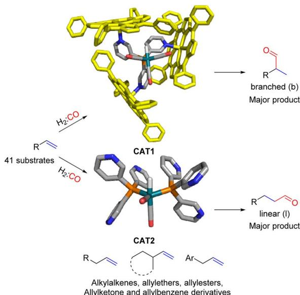
Scheme 1 Substrate scope investigation of the encapsulated  $[\text{Rh}(\text{H})(\text{CO})_3(\text{P}(\text{mPy}_3)(\text{ZnTPP})_3)]$  catalyst (CAT1) in the hydroformylation reaction of terminal alkenes.
