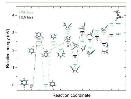
Fig. 5 Potential energy surface for the fragmentation to methylene-cyclopropene. † from pyridine<sup>\*+</sup> leading to either HCN loss (C-pathway, black pathway) or HNC loss (iCpathway, green pathway). The energies are calculated at the B3LYP-GD3/N07D level of theory and are corrected for the zero-point vibrational energy.
