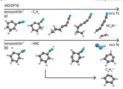
Fig. 8 Exemplary pathways for loss of (a)  $C_2H_4$  and (b) HNC from canonical benzonitrile as observed in the MD/DFTB simulations at 8.8 eV internal energy of the respective cation using Set1 parameters. The arrows indicate time.
