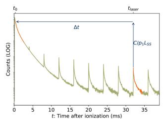
Fig. 5 Graphical example of method for determining back-shifted times  $t_0$  by fitting the laser-induced dissociation rate  $R_{\rm e}(t_{\rm after})$  to the spontaneous dissociation rate of source-heated ions R(t). In this example,  $t_{\rm laser}=32$  ms and  $t_0=320$   $\mu s$ .
