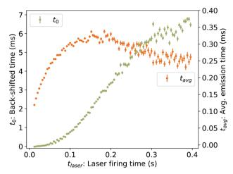
Fig. 6 (Left axis) Back-shifted times  $t_0$  to which the vibrational energy distribution is reheated following photon absorption at time  $t_{\rm laser}$ , determined from laser-induced decay curves  $R_{\rm e}(t_{\rm after})$ . (Right axis) Average emission times  $t_{\rm avg}$ .
