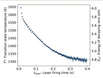
**Fig. 8** Transition state temperatures  $T^{\ddagger}$  (left axis) and corresponding vibrational energies  $E_{\rm m}$  (right axis) of ions decaying following photon absorption at time  $t_{\rm laser}$ , determined from KER distributions  $P_{\rm e}(\varepsilon)$ .
