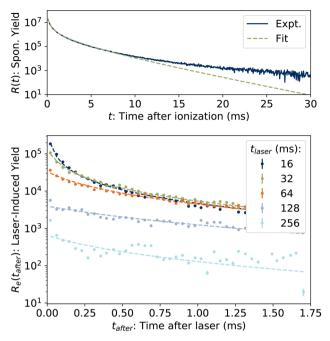
Fig. 2 (Top) Spontaneous dissociation rate R(t), fit of eqn (4). (Bottom) Examples of laser-induced dissociation rates  $R_{\rm e}(t_{\rm after})$  with fits of eqn (8).
