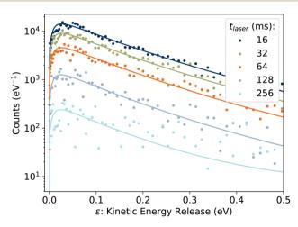
Fig. 7 Examples of KER distributions  $P_{\rm e}(\varepsilon)$  resulting from dissociation of laser-excited 1-CNN<sup>+</sup>. Solid lines are fits to eqn (9).
