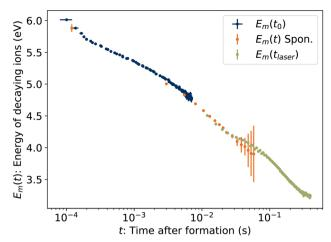
Fig. 10 Energies  $E_m$  of ions decaying at time t. Blue symbols  $E_m t_0$  are the energies from Fig. 8 plotted against the back-shifted time  $t_0 + t_{avg}$ . The green symbols  $E_m(t_{laser})$  give the energy in eqn (15) as a function of laser firing time. The orange symbols  $E_m(t)$  are the energies of spontaneously decaying 1-CNN<sup>+</sup> determined previously.<sup>6</sup>
