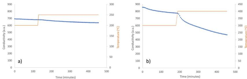
Fig. 9 Ammonia production reaction profiles of  $\text{Ni}_3\text{CuN}$  reacted with  $60 \text{ mL min}^{-1}$  of 3 : 1  $\text{H}_2/\text{N}_2$  (a) for 2 hours 5 minutes at  $200^\circ\text{C}$  and 5 hours 25 minutes at  $250^\circ\text{C}$  and (b) for 3 hours at  $300^\circ\text{C}$  and 4 hours 25 minutes at  $400^\circ\text{C}$ .
