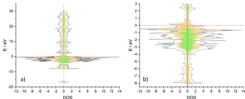
Fig. 14 Plots for the projected density of states (DOS) for  $\text{Ni}_3\text{CuN}$ : (a) full DOS and (b) highlighted area for metal d states at the Fermi level. Black lines: total DOS, shaded orange: Ni and shaded green: Cu.
