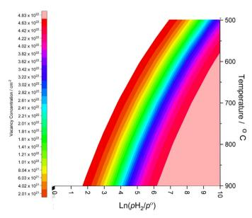
Fig. 3 Surface N vacancy concentration as a function of  $H_2$  partial pressure (where  $p^{\circ}$  is ambient pressure) and temperature, as estimated from *ab initio* thermodynamics.
