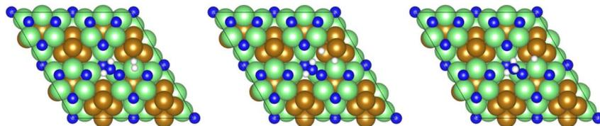
Fig. 6 Graphics illustrating the initial (left), transition (centre), and final (right) state geometries associated with hydrogenation of the  $N_2H_2^{\square}$  intermediate to yield the  $N_2H_3^{\square}$  intermediate (Table 2, process 4).
