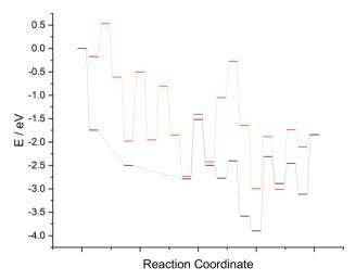
Fig. 17 Computed reaction profile for the two mechanisms for ammonia synthesis on  $Fe_3Mo_3N$ , for the associative Eley–Rideal–Mars–van-Krevelen mechanism (black) and the dissociative Langmuir–Hinshelwood mechanism (red).
