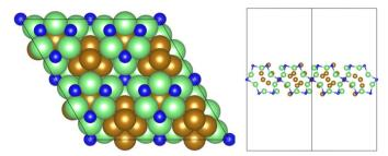
Fig. 1 Graphic illustrating the symmetric, non-stoichiometric thin-film slab model used to model the  $Fe_3Mo_3N$  surface, from the top (left) and side (right), as viewed across the cell diagonal. The pristine surface is illustrated, *i.e.* no N vacancies are present. Key: green, Mo; brown. Fe: blue. N.
