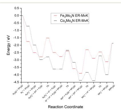
Fig. 18 Computed reaction profiles comparing the ER–MvK mechanism for ammonia synthesis on  $Fe_3Mo_3N$  (red) and for  $Co_3Mo_3N$  (black).<sup>35</sup>
