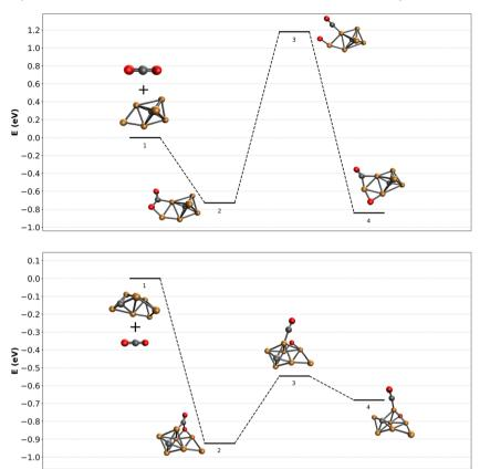
Fig. 7 Reactive potential energy surface for CO<sub>2</sub> dissociation over the lowest energy structures found for  $Cu_6C^-$  and  $Cu_7C^-$ , calculated at the TPSSh/def2-TZVPD level of theory. Energies (in eV) are given with respect to the bare clusters and free CO<sub>2</sub>.
