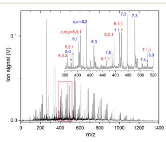
Fig. 2 Mass spectrum of the products formed when reacting anionic  $Cu_nC_m^-$  clusters with  $CO_2$ . Mass peaks in the inset are labeled by (n and m) or (n, m, and p) for  $Cu_nC_m(CO_2)_p^-$ .
