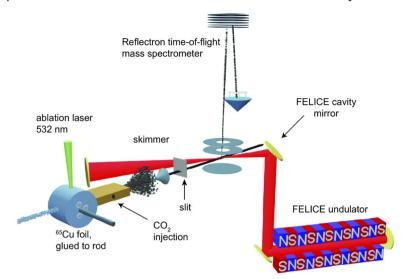
Fig. 1 Schematic of experimental setup.
