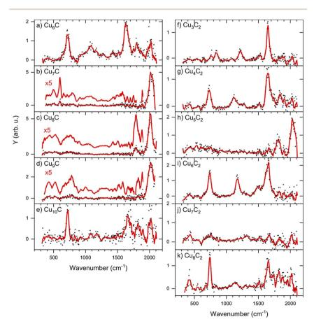
**Fig. 3** IRMPD spectra of  $[Cu_nC \cdot CO_2]^-$  (left) and  $[Cu_nC_2 \cdot CO_2]^-$  (right). The red lines are five-point adjacent-averages of the solid dots.
