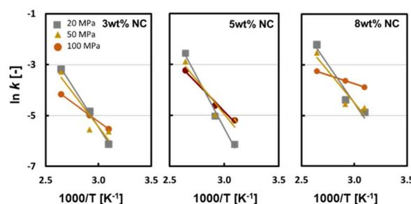
Fig. 12 Arrhenius plots of the degradation rate constant at 50, 70, and 105 °C. The powders were prepared at □: 20 MPa, △: 50 MPa, and ○: 100 MPa. (Yoshii *et al.*, 2023)<sup>46</sup> "Reproduced from ref. 46 with permission from Taylor and Francis, copyright 2023".
