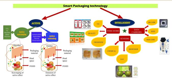
Fig. 2 Schematic representation of smart packaging technology.
