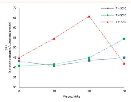
Fig. 2 Effect of the PEF energy input and temperature on the maximum soluble protein extraction yield  $(1/K_2)$  for ground particles (blue square – T = 30 °C; green circle – T = 50 °C; red triangle – T = 70 °C).
