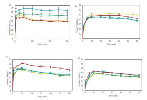
Fig. 1 Extraction kinetics of soluble proteins from nettle leaves: (a) 70 °C (<1 mm), (b) 70 °C (<3 mm), (c) 50 °C (<1 mm), and (d) 50 °C (<3 mm), from 0 to 30 kJ kg $^{-1}$  of specific energy (yellow triangle – control; green circle – 10 kJ kg $^{-1}$ ; blue square – 20 kJ kg $^{-1}$ ; red rhombus – 30 kJ kg $^{-1}$ ).
