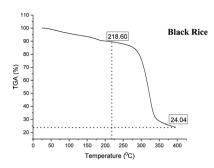
Fig. 4 Thermogravimetric analysis (TGA).
