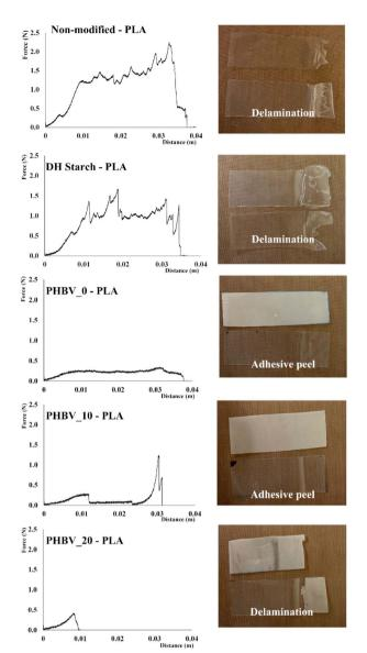
Fig. 3 Typical behaviour of the seal profile and the image of the separation mode of the different bilayers (non-modified starch-PLA, DH starch-PLA, PHVB\_0-PLA, PHVB\_10-PLA and PHVB\_20 PLA) during the sealing strength test
