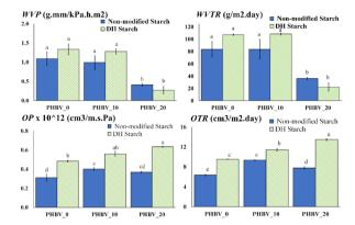
Water vapour permeability (WVP), water vapour transmission rate (WVTR), oxygen permeability (OP) and oxygen permeability transmission rate (OPTR) for tri-layer materials. Means with different letters are significantly different (p < 0.05).
